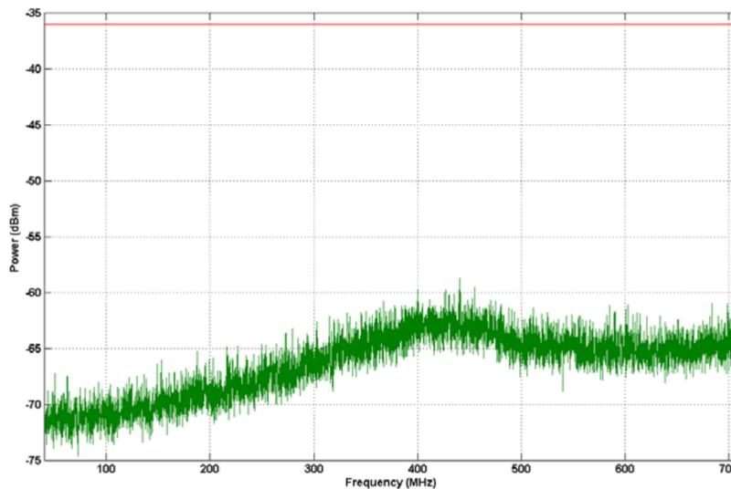
**Figure 20. Spurious Emission 40 MHz - 710 MHz**
