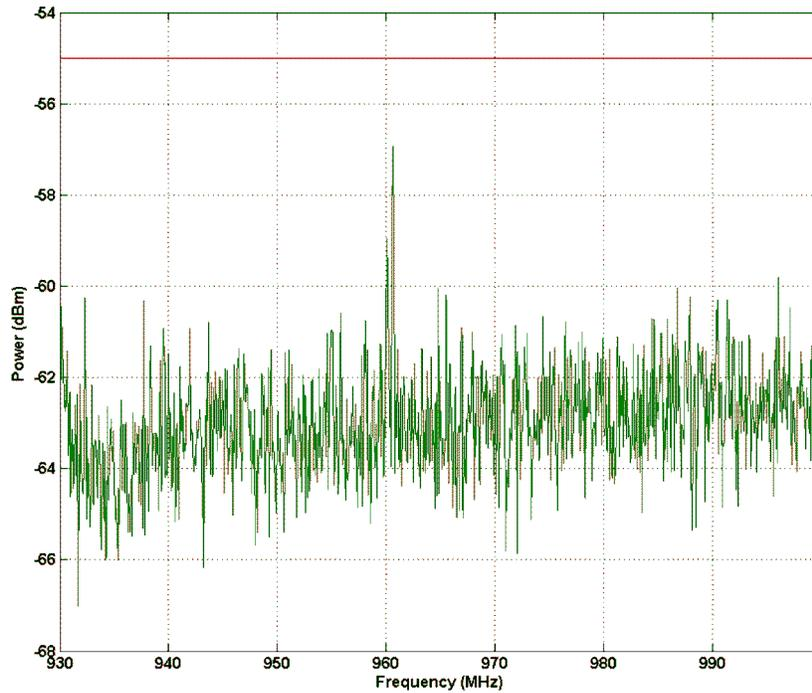
**Figure 17. Spurious Emission 930 MHz - 1000 MHz**
