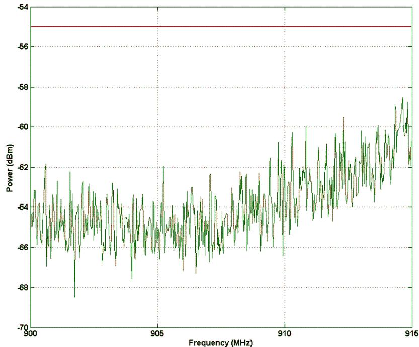
**Figure 6. Spurious Emission 900 MHz - 915 MHz**
