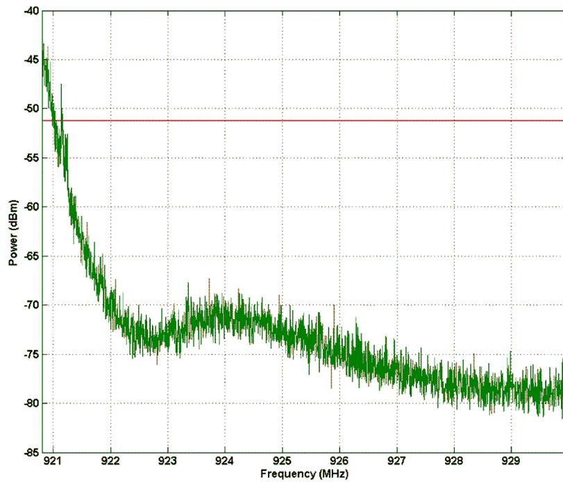
**Figure 24. Spurious Emission 920.8 MHz - 930 MHz**
