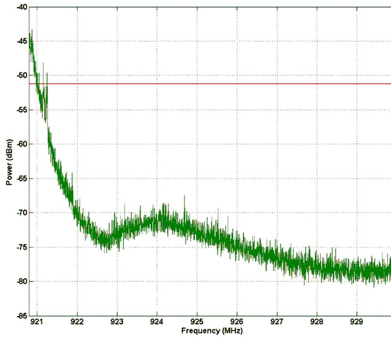
**Figure 16. Spurious Emission 920.8 MHz - 930 MHz**
