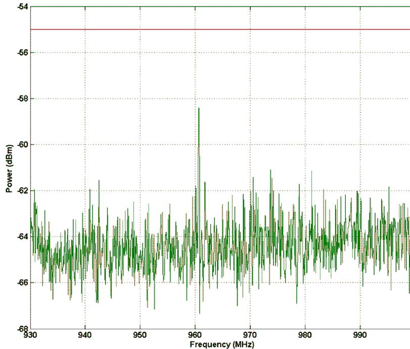
**Figure 9. Spurious Emission 930 MHz - 1000 MHz**
