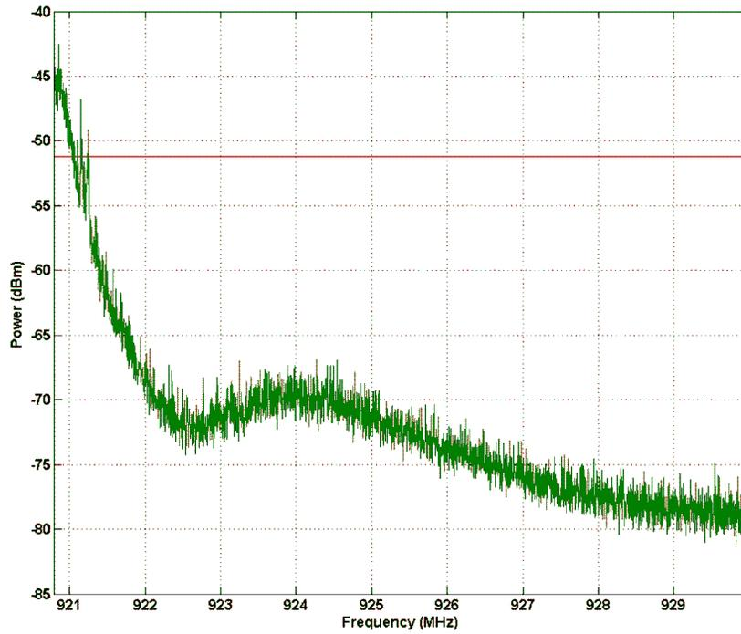
**Figure 8. Spurious Emission 920.8 MHz - 930 MHz**
