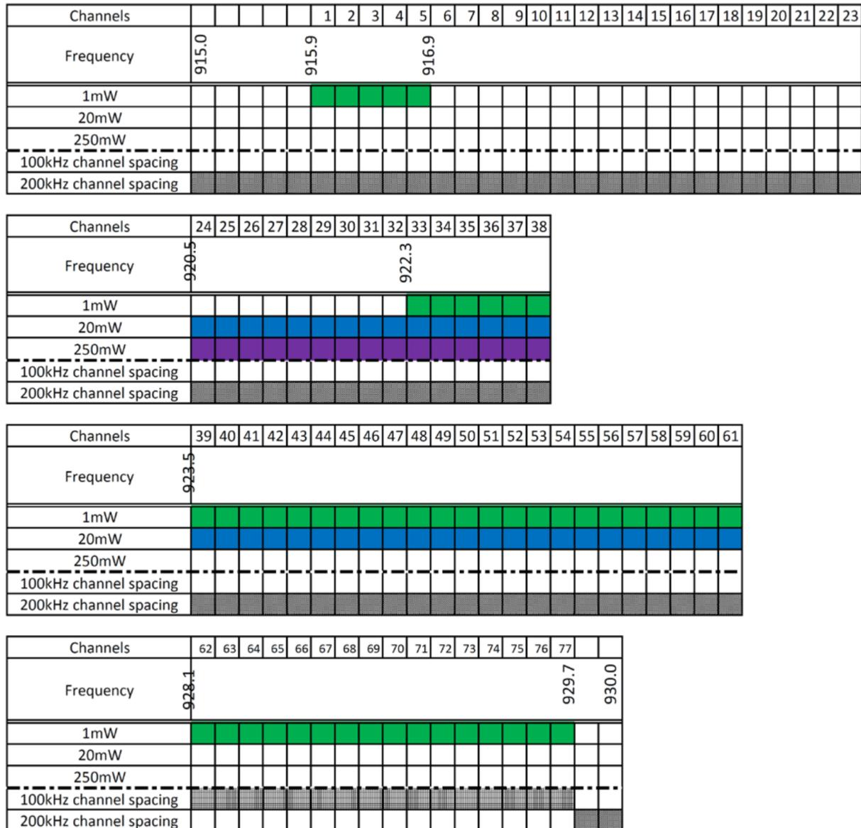
Figure 3. Channel Plan for 920 MHz Band Radio Equipment
