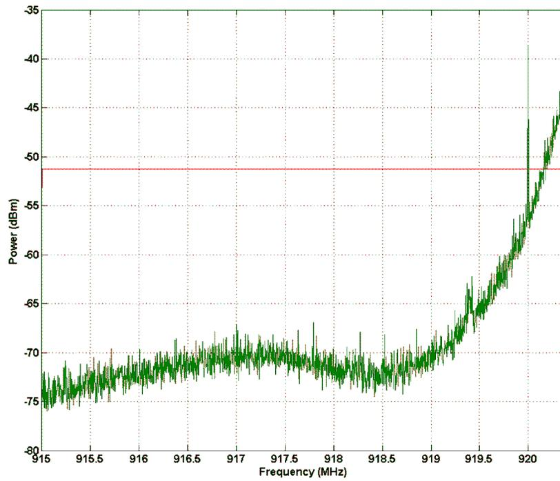
**Figure 7. Spurious Emission 915 MHz - 920.4 MHz**
