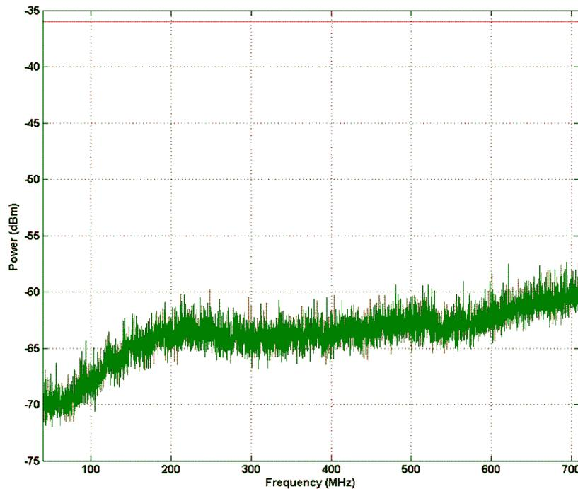
**Figure 4. Spurious Emission 40 MHz - 710 MHz**
