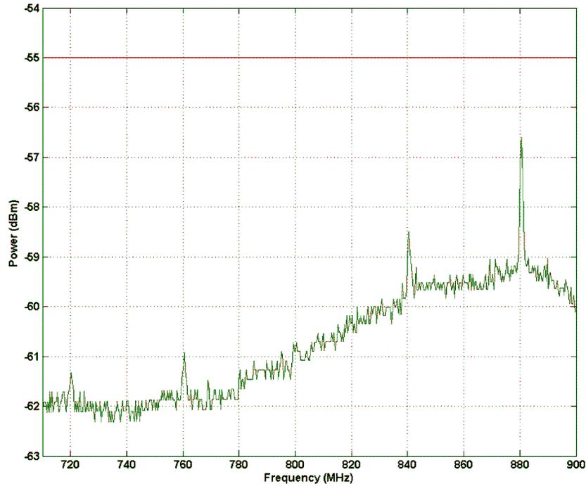
**Figure 13. Spurious Emission 710 MHz - 900 MHz**
