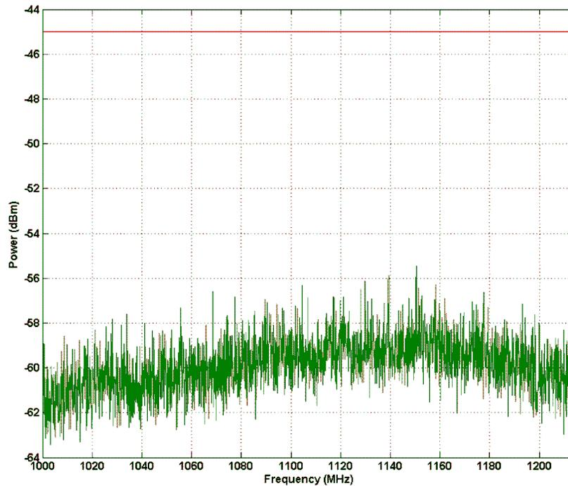
**Figure 18. Spurious Emission 1000 MHz - 1215 MHz**
