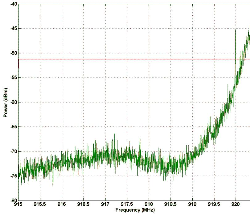
**Figure 23. Spurious Emission 915 MHz - 920.4 MHz**
