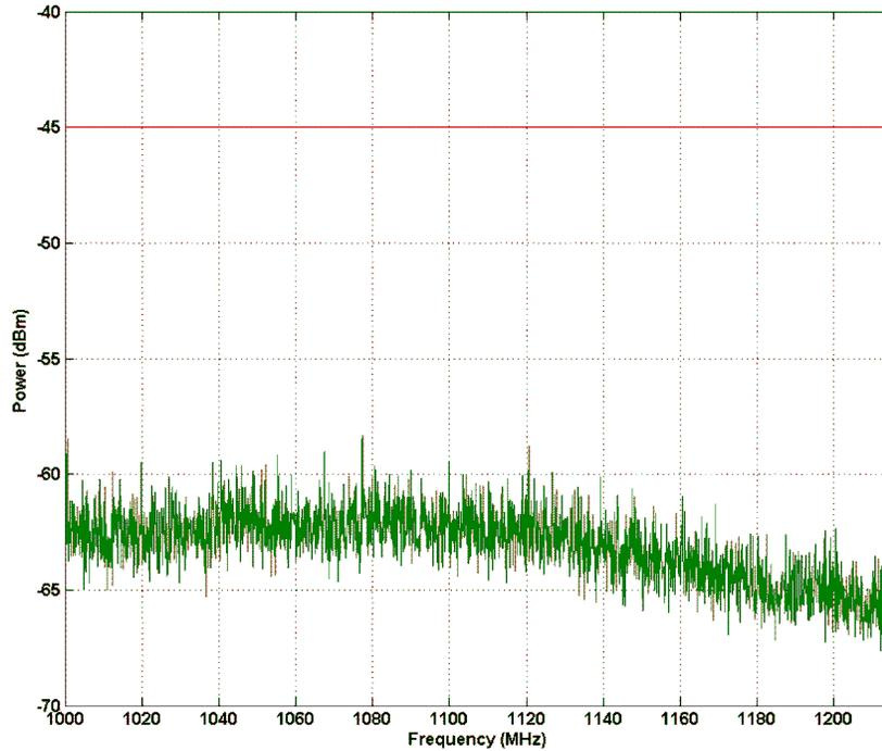
**Figure 10. Spurious Emission 1000 MHz - 1215 MHz**
