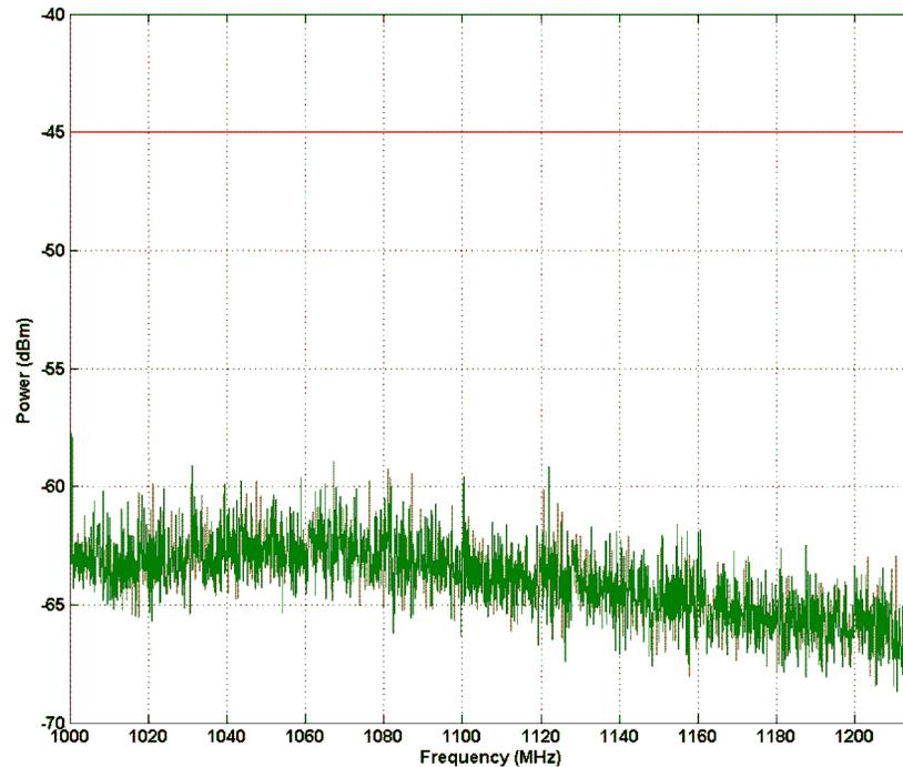
**Figure 26. Spurious Emission 1000 MHz - 1215 MHz**
