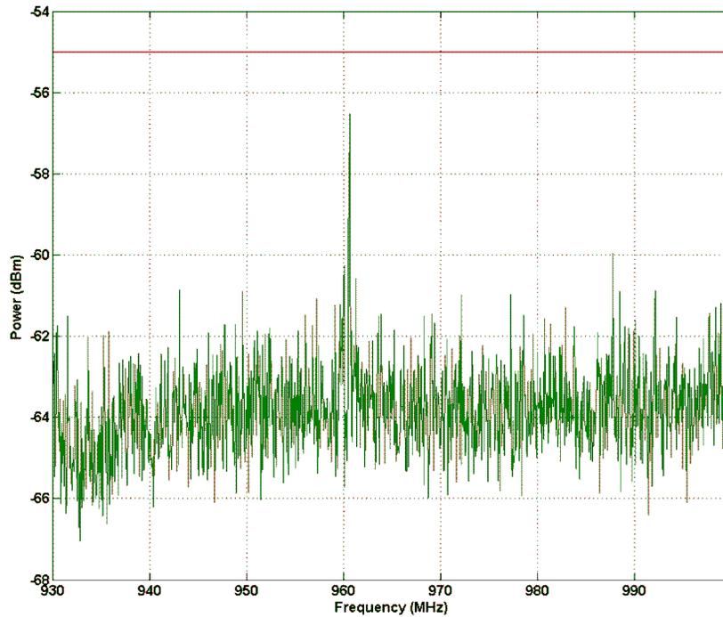
**Figure 25. Spurious Emission 930 MHz - 1000 MHz**
