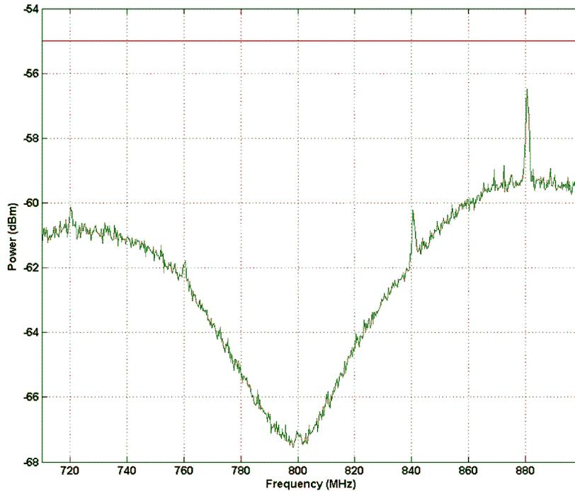
**Figure 21. Spurious Emission 710 MHz - 900 MHz**
