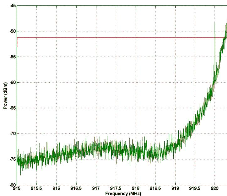
**Figure 15. Spurious Emission 915 MHz - 920.4 MHz**
