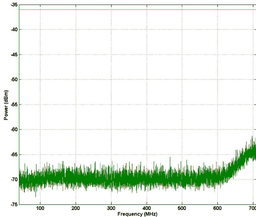
**Figure 12. Spurious Emission 40 MHz - 710 MHz**
