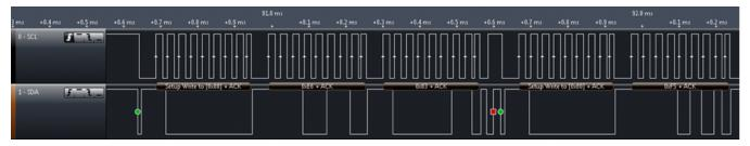
Figure 20. I2C Set Up and Start Humidity Measurement
