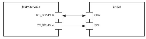
Figure 2. Block Diagram of Interface Between MSP430F2274 and SHT21
