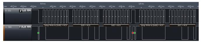
Figure 18. I2C Set Up and Start Temperature Measurement
