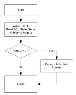
Figure 9. PUSH Interrupt Service Routine
