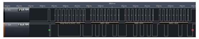
Figure 21. I2C Read Humidity Measurement Results
