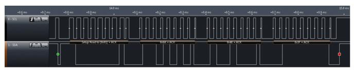
Figure 19. I2C Read Temperature Measurement Results
