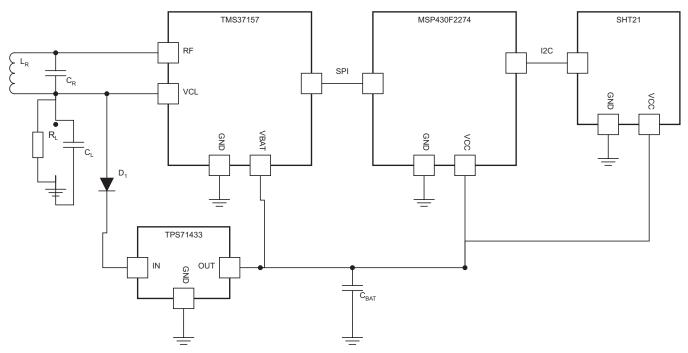
Figure 3. Principle Schematic of the Wireless Sensor
