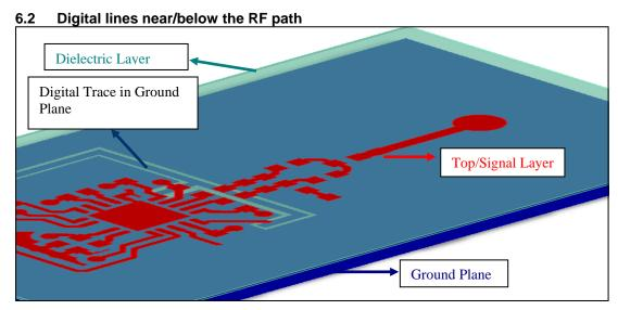
Figure 6: Digital Lines directly below the RF path
