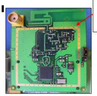
RF Shield (vias from top ground to ground plane)
