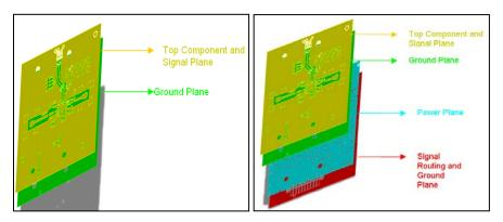
Figure 1: A two layer board stack-up. Figure 2: A four layer board stack-up
