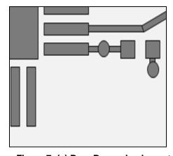
Figure 7: (a) Poor Bypassing Layout
