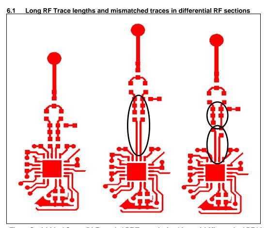
Figure 5: (a) Ideal Case (b) Extended RF Transmission Lines (c) Mismatched RF Lines
