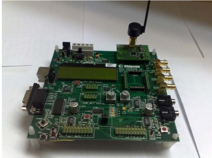
Figure 3. SmartRF04EB with CC2510EM
