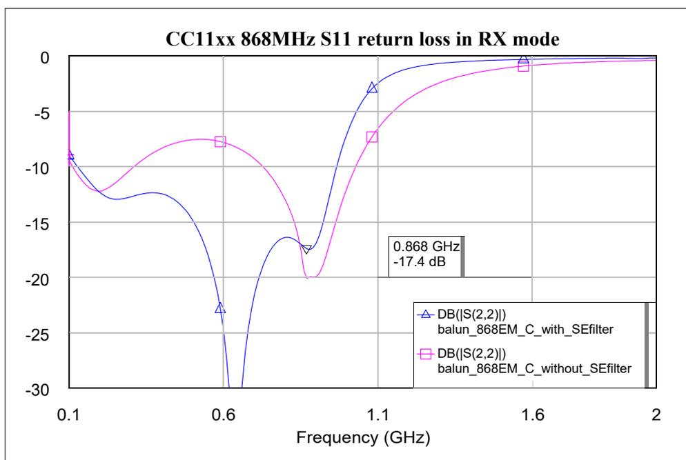
**Figure 4. Return Loss at the Antenna Port**
