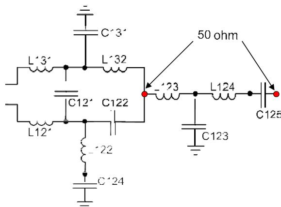
Figure 2. 50 Ohm Points in the Filterbalun
