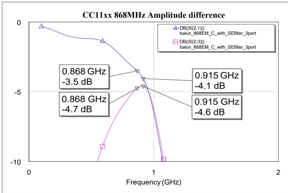
Figure 7. Amplitude Difference
