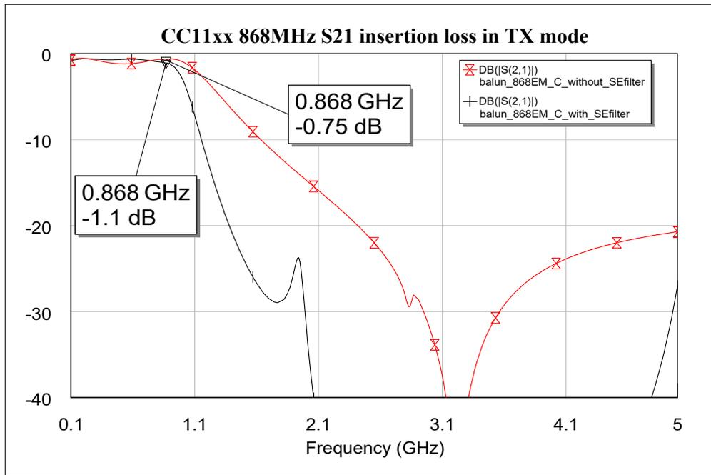
**Figure 6. Insertion Loss**
