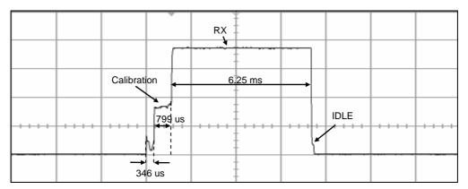
Figure 10. Current Consumption (EVENT1 = 3 and RX Timeout = 6.25 ms)
