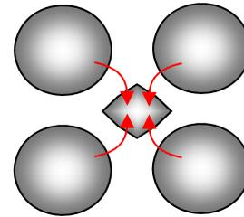
Memory Dip too fast + paste suppress by 4 balls and extrude the additional paste up & attached on the bottom of substrate surface.
