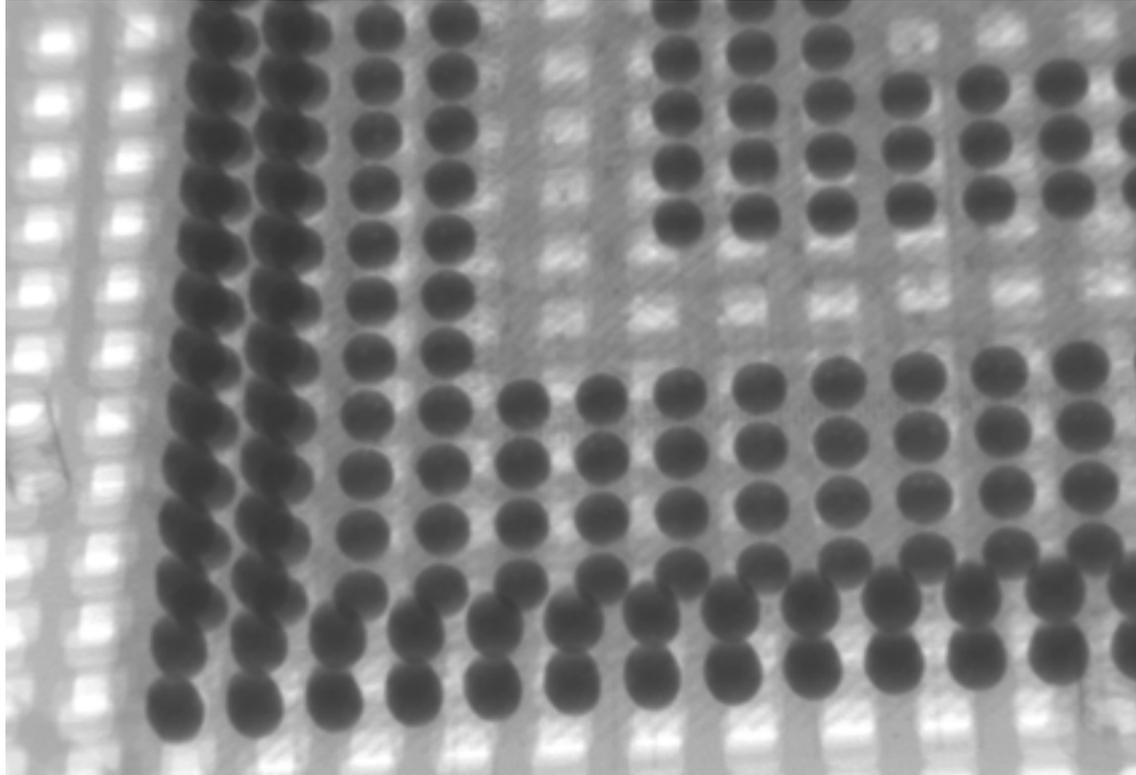
Picture: Memory mounted by solder paste, SMD board, After reflow.
