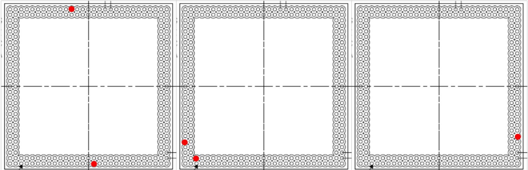
**Defect:** Random single or double non-wet solder joints
