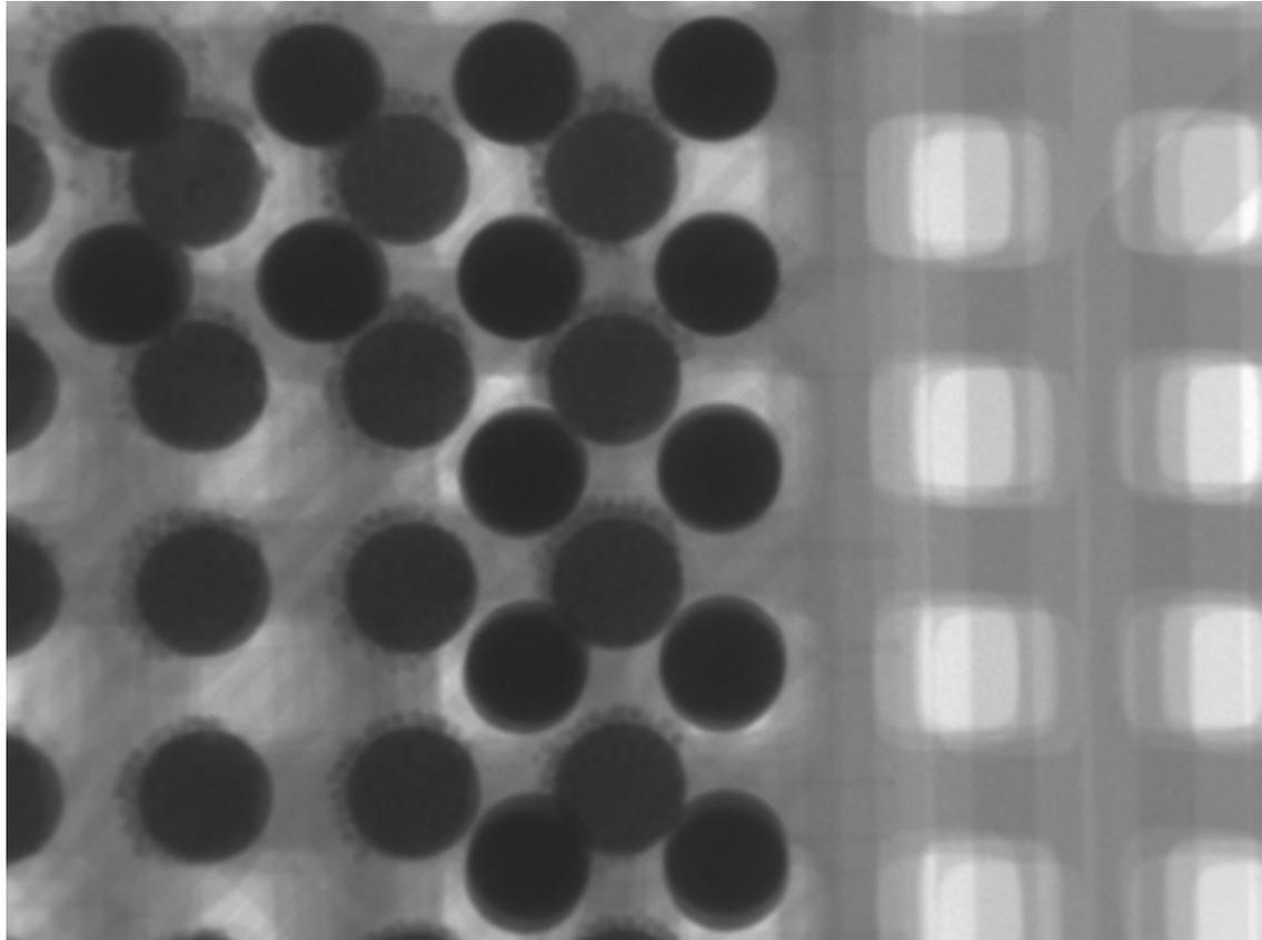
Picture: POP and Memory mount on PCB. Before reflow.
