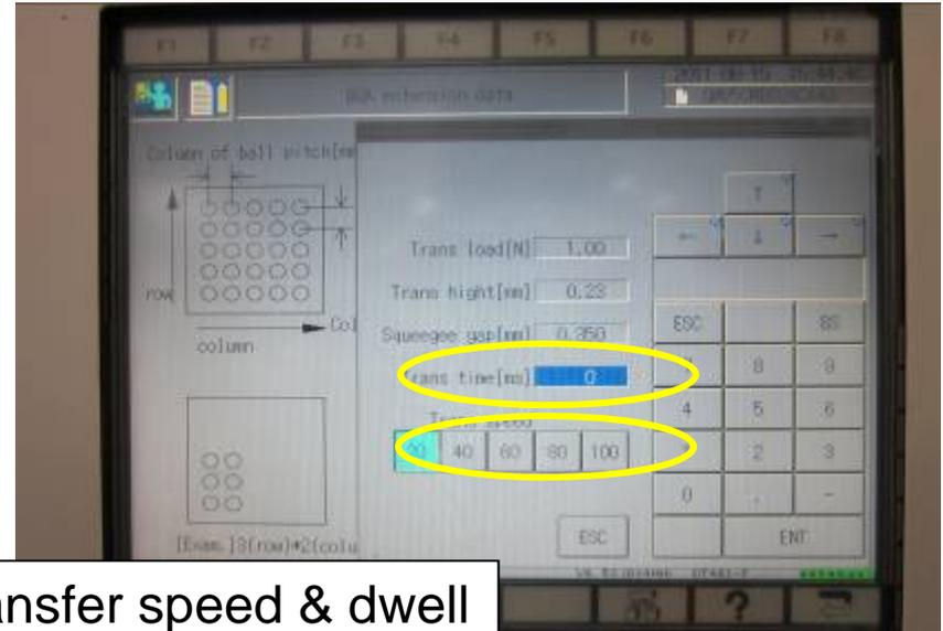
Balance the in/out transfer speed & dwell time to get optimized solder dipping.
