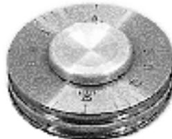
A hardened and ground double wheel with an eccentric cam in the middle is rolled over a newly applied film. The wetting line on the middle cam is read off on a scale as wet film thickness. Total measuring range: 1500 microns, available in 8 different sub-ranges.
