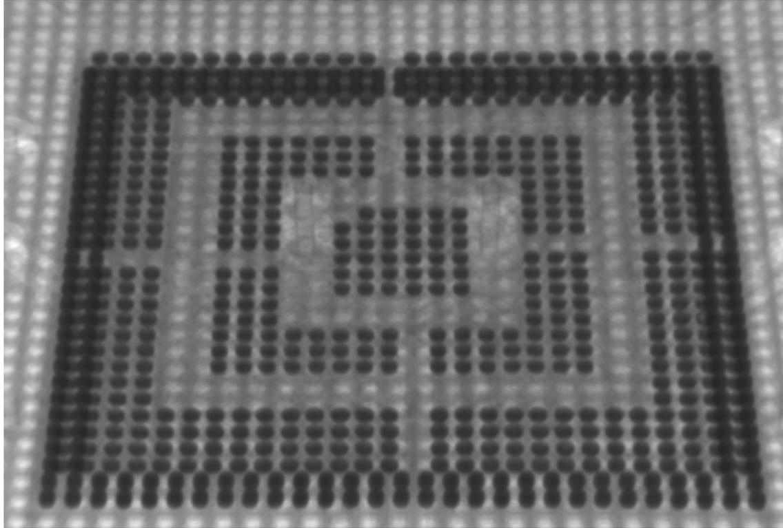
Picture: Memory mounted by flux, SMD board, After reflow
