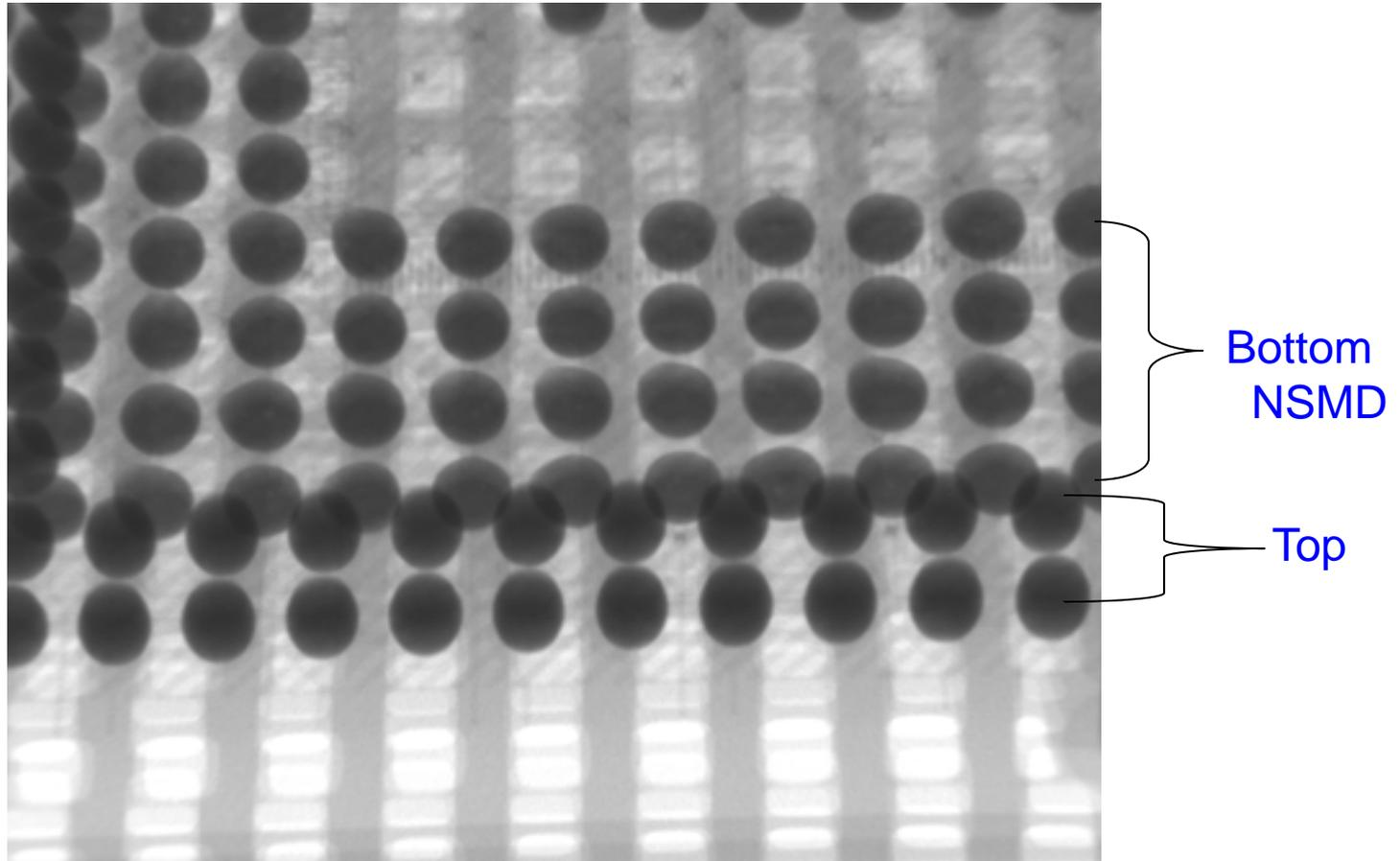
Picture: Memory mounted by flux, NSMD board, After reflow
