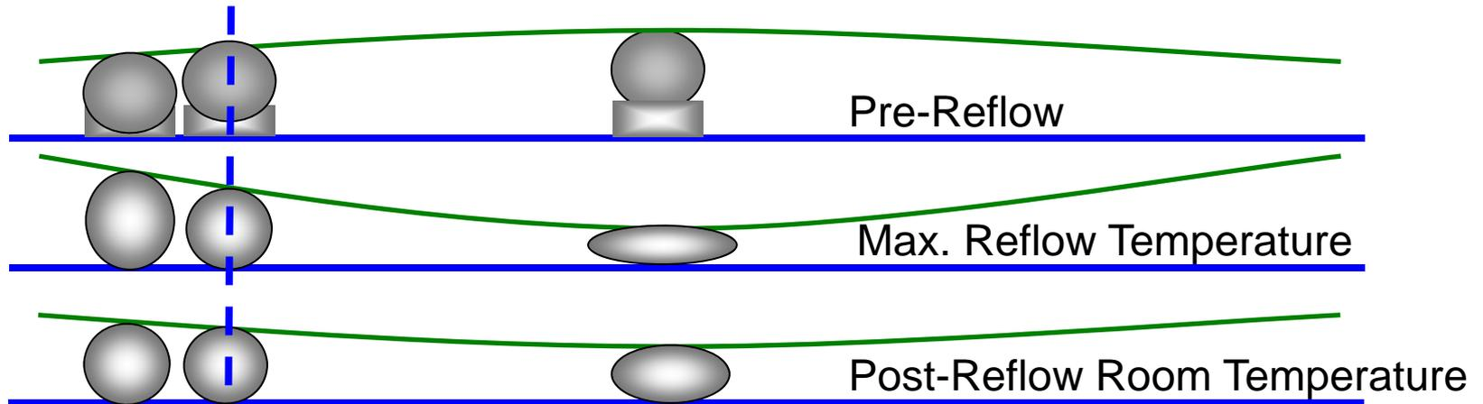
Neutral solder ball at maximum reflow temperature (nominal height)
