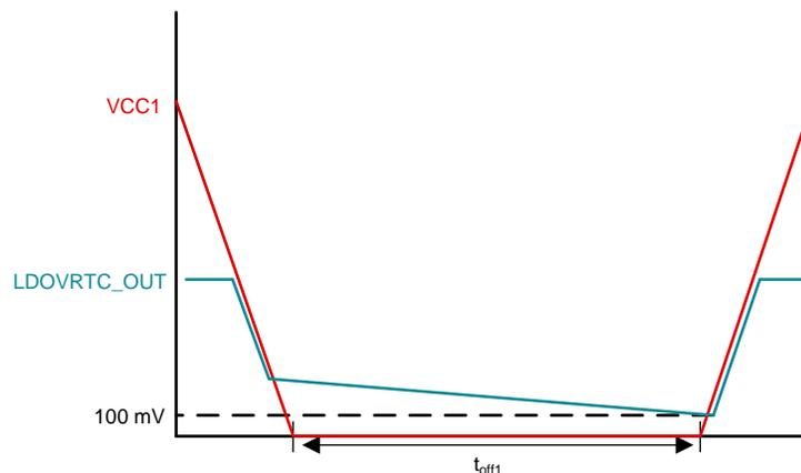
Figure 3. LDOVRTC Discharge With No Resistor
