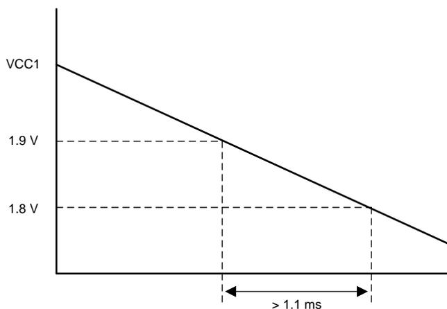
Figure 1. VCC Falling Profile
