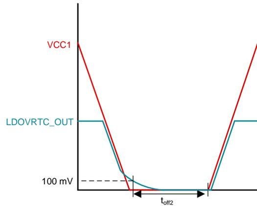
**Figure 4. LDOVRTC Discharge With Resistor**
