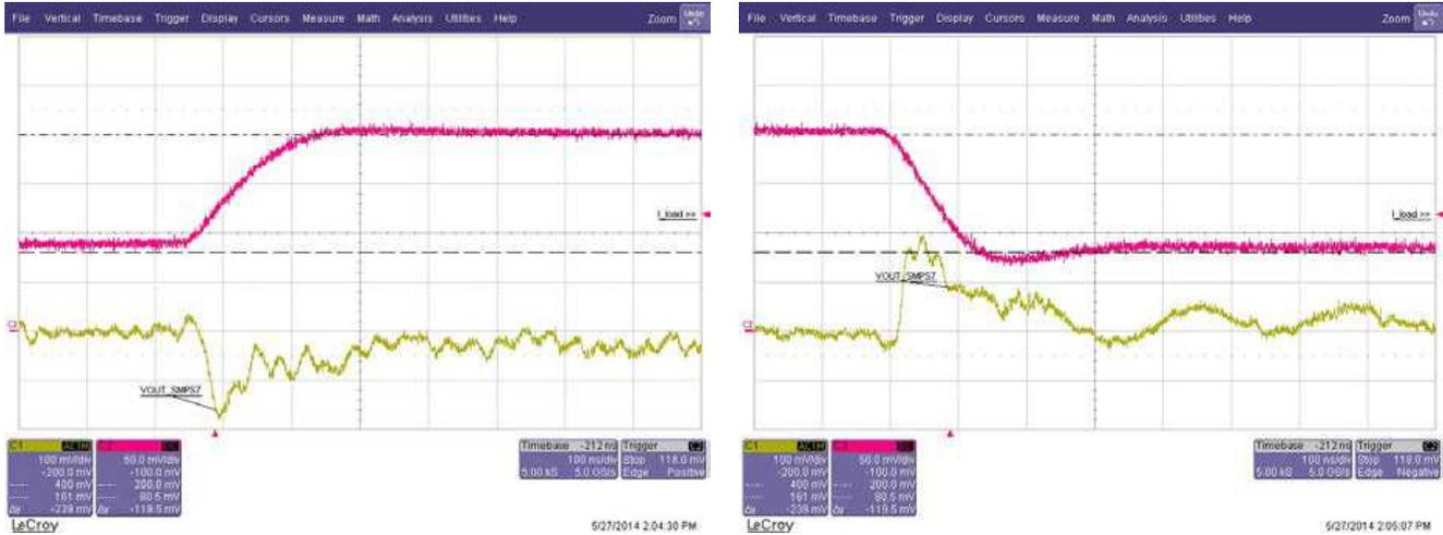
Figure 8. Single-Phase Load-Step Response 5-V Input, 1.05-V Output, 94  $\mu$ F, Hot
