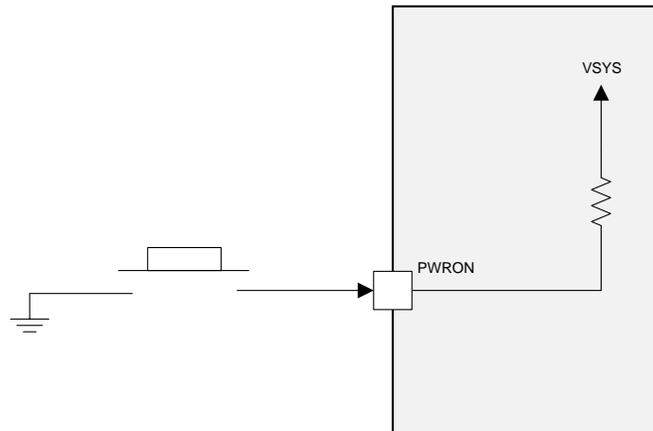
**Figure 2. Typical PWRON Configuration**
