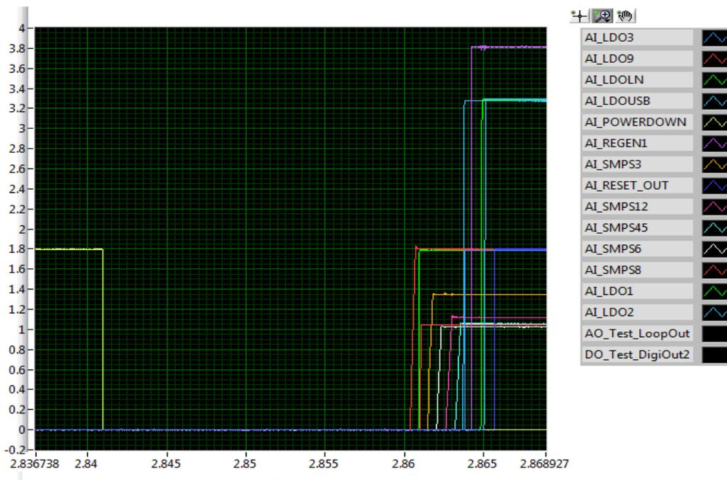
Figure 10. POWERDOWN as a Gating Condition
