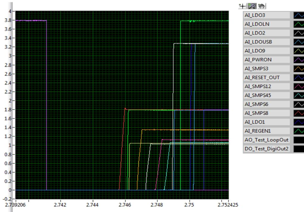
**Figure 3. ON Request Using PWRON**
