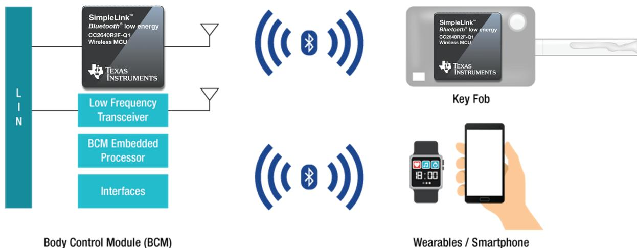
**Figure 2.** Bluetooth low energy-enabled car access block diagram.
