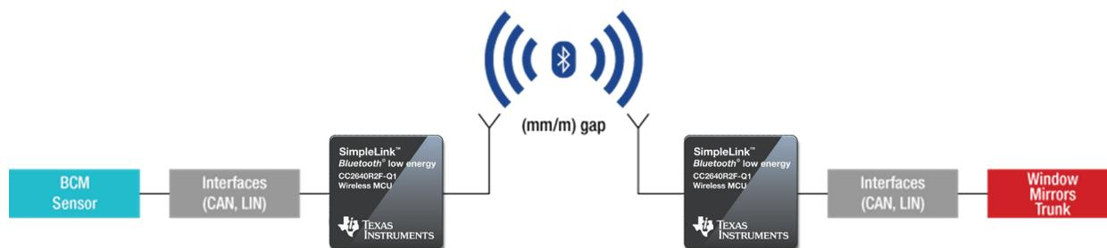
**Figure 3.** Bluetooth low energy-enabled cable replacement concept.
