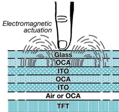
**Figure 5.** ITO capacitive-touch sensor with TFT LCD.
