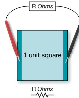
**Figure 6.** Sheet resistance for one unit square.
