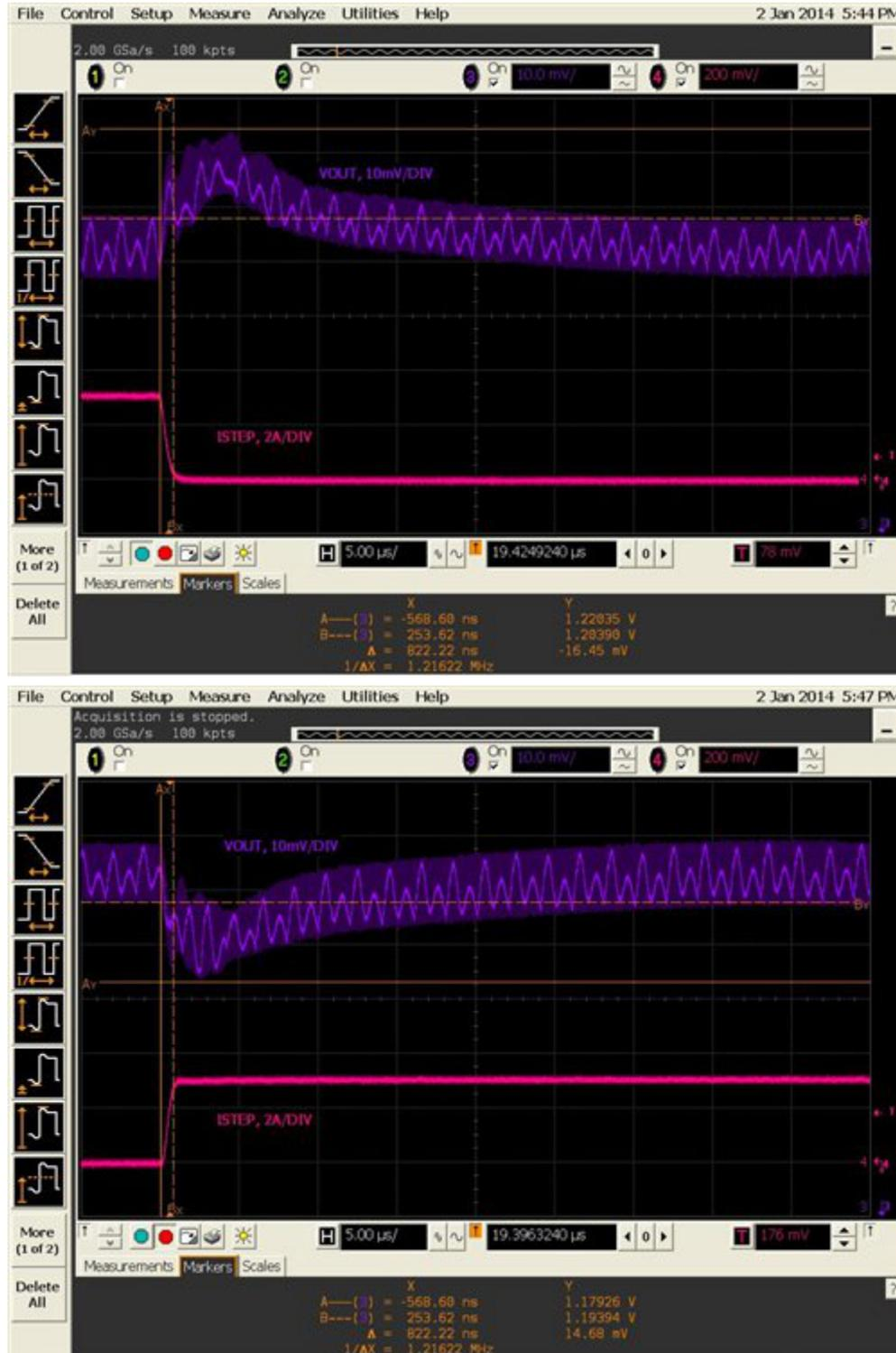
Figure 5. Load transient response of the TPS53319 (Vout = 1.2V)
