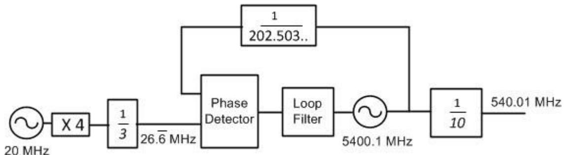
Figure 2. Avoiding Integer Boundaries Using a Programmable Multiplier
