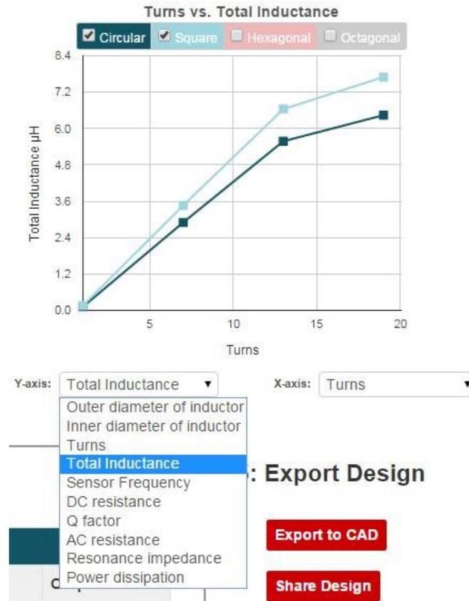
Figure 6. Output Parameters Plotted against Input Parameters and Compared to Different Coil Types
