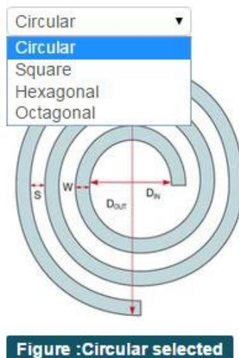
**Figure 3. WEBENCH Coil Designer Supports Circular, Hexagonal, Octagonal and Square Coil**
