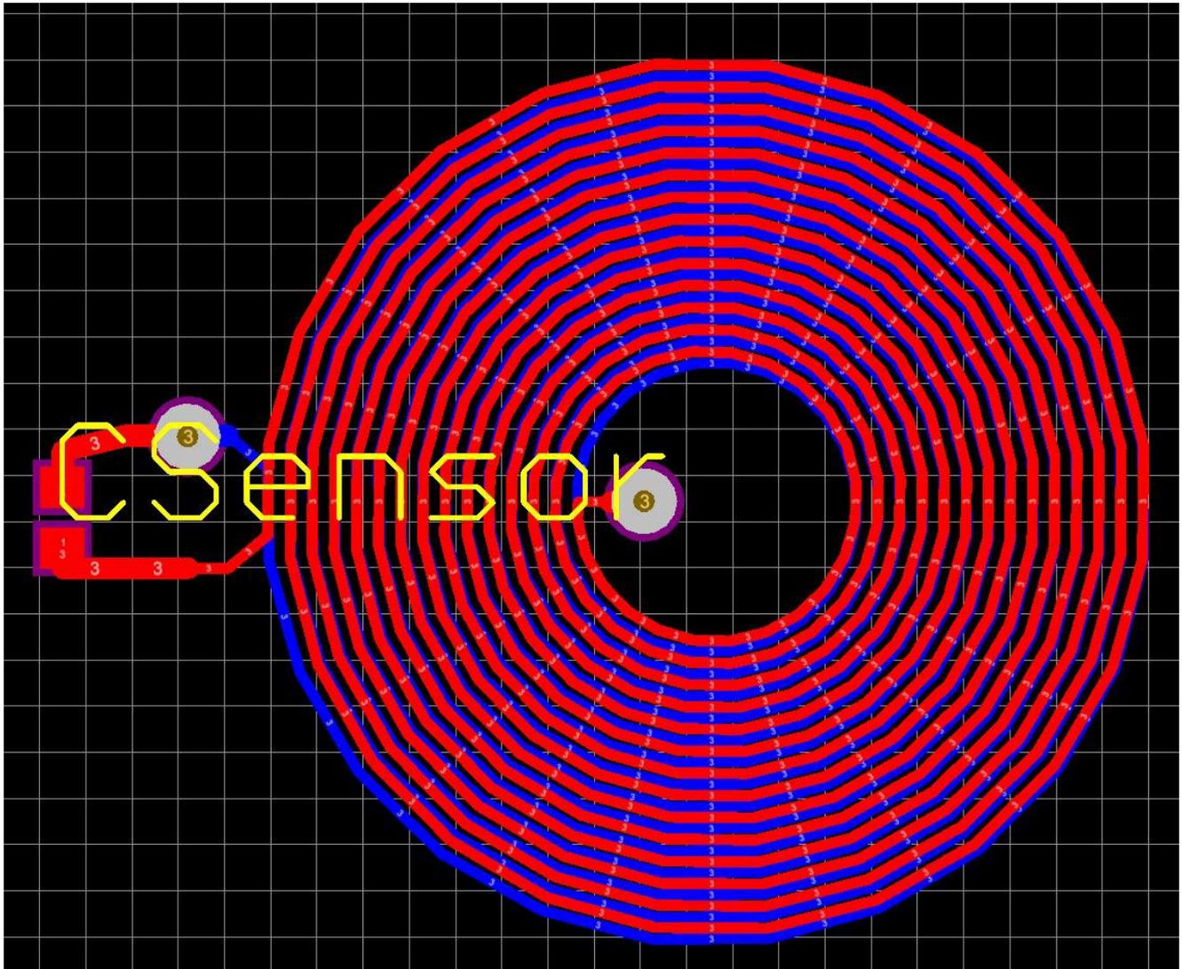
**Figure 8. The Resulting Sensor Coil When Imported into Altium Designer**
