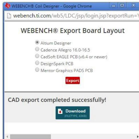
Figure 7. The Export Function Exports the Coil into PCB Layout Software
