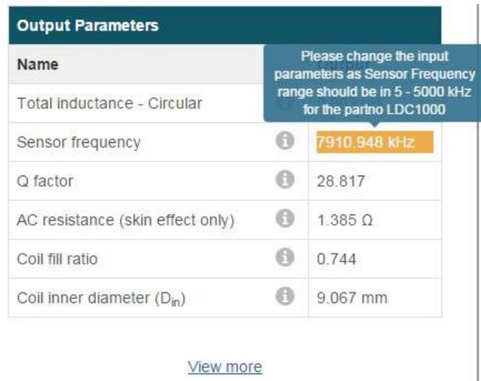
**Figure 5. Designing an 8MHz Sensor for the LDC1000 Produces a Warning and Recommendation for Avoiding the System Constraint**
