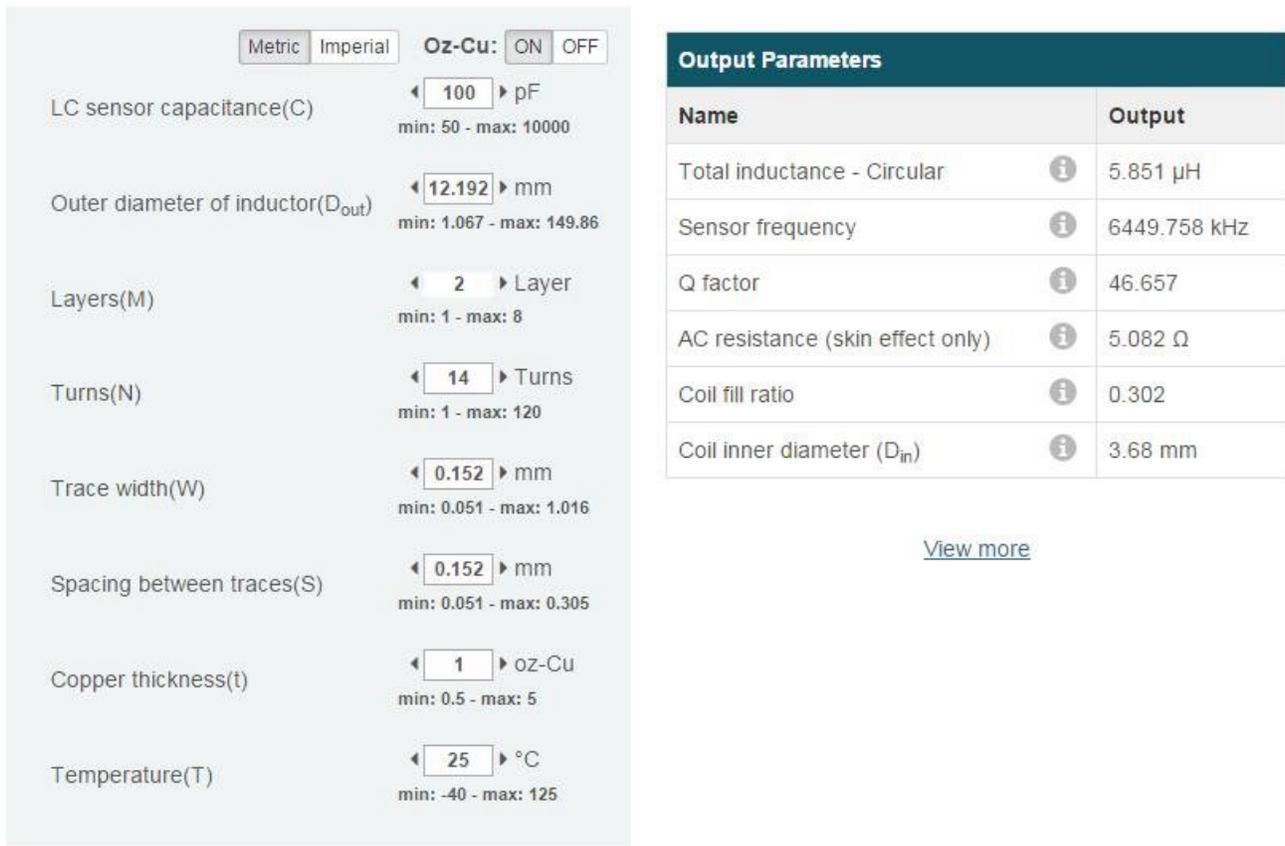
**Figure 4. Output Parameters for Given Coil Geometries. Clicking ‘View More’ Displays Advanced Output Parameters**
