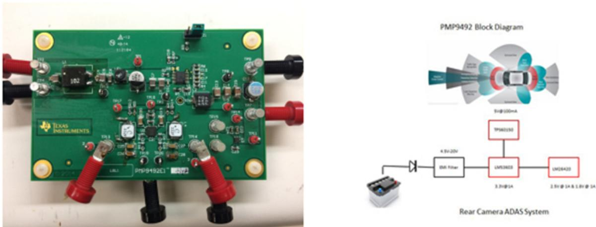
**Figure 3.** TI's [CISPR 25 class 5 multi-output reference design for automotive rear camera and ADAS systems](#).
