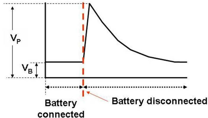
Figure 2. Diagram of a Load Dump Condition.
