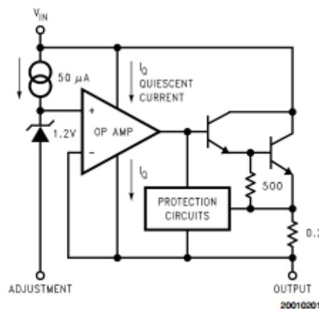
**Figure 1. LM317-N Functional Schematic**
