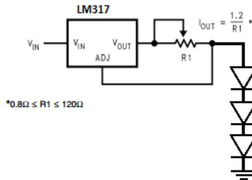
Figure 3. Constant-current LED Driver Using the LM317-N
