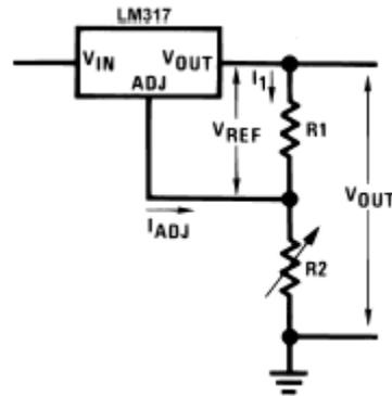
Figure 2. Typical Application Using the LM317-N
