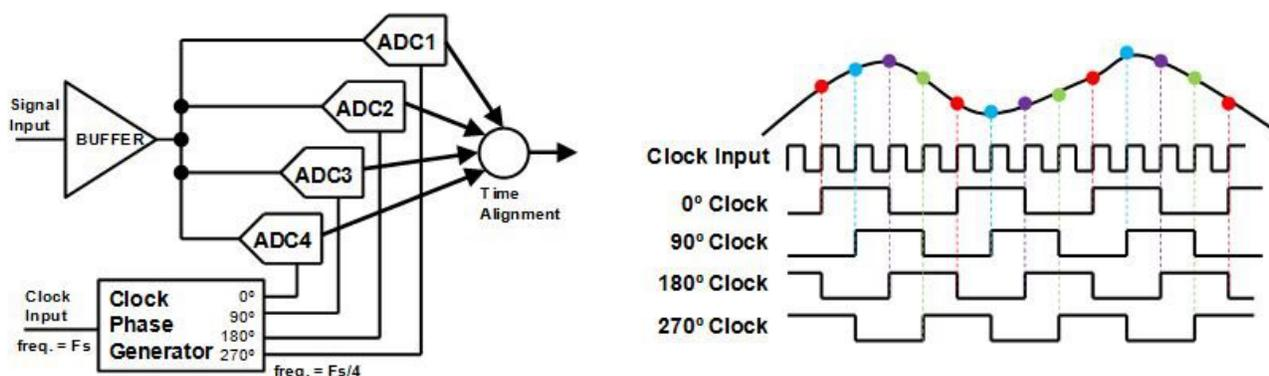
**Figure 1. Four-way Interleaving Block Diagram and Timing Chart**
