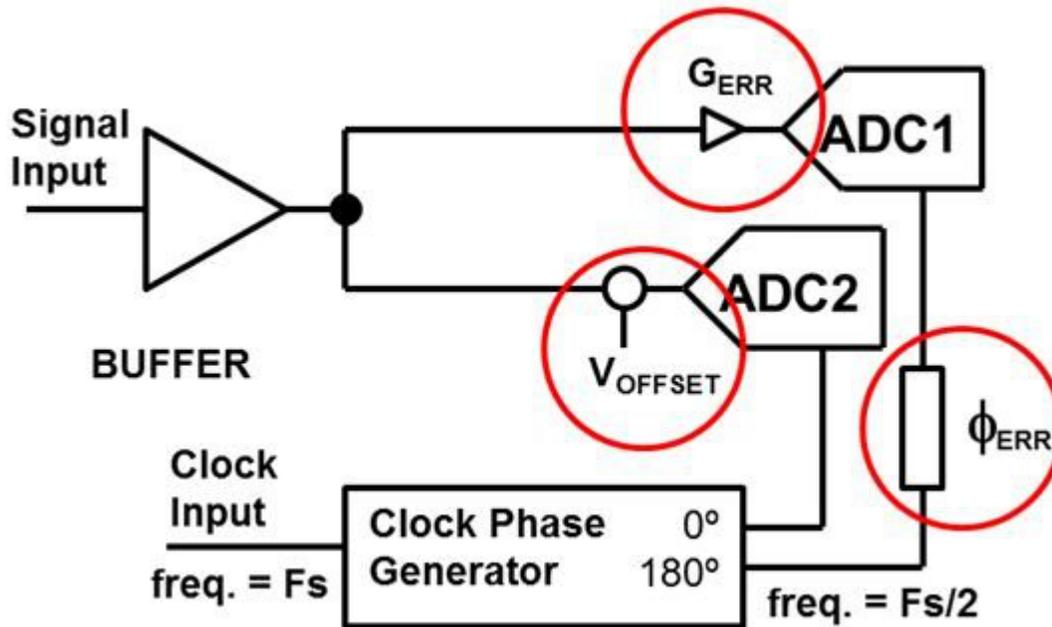
**Figure 2. Sources of Error in an Interleaved ADC**
