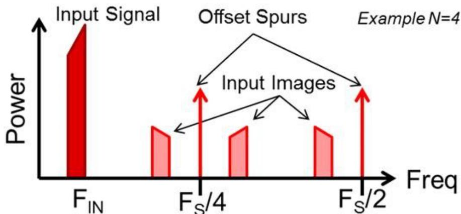
**Figure 3. Interleaving Spurious for a Four-core Device**
