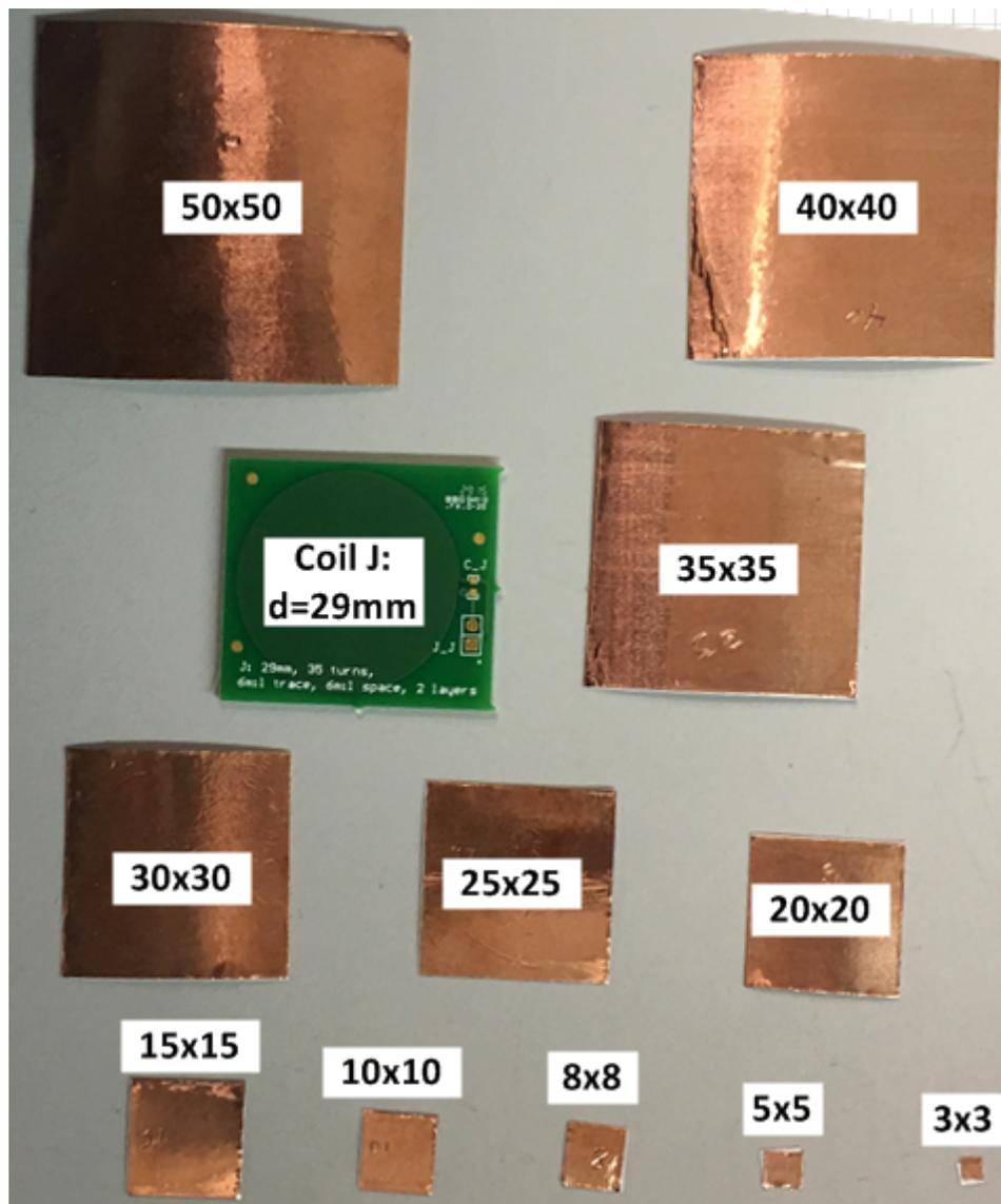
Figure 1. Conductive Targets Made from Copper Tape (All Sizes in Millimeters)
