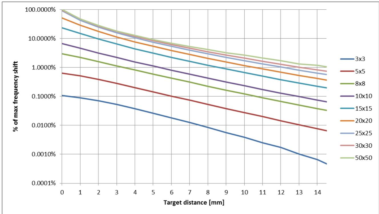
**Figure 3. Percentage of Maximum Frequency Shift vs. Target Distance (in Millimeters)**
