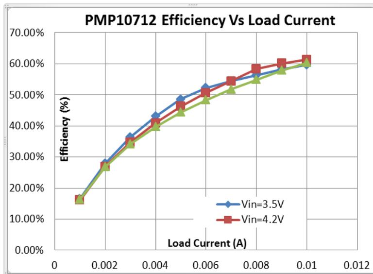
**Figure 2. Efficiency Using the LM3481 Boost Controller**
