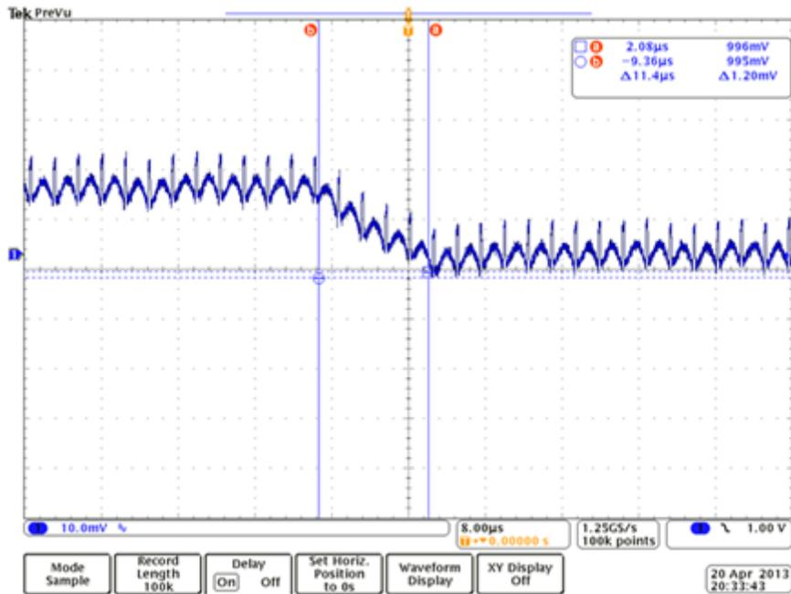
Figure 5. Output-voltage Change (AVS) via the PMBus VOUT\_COMMAND
