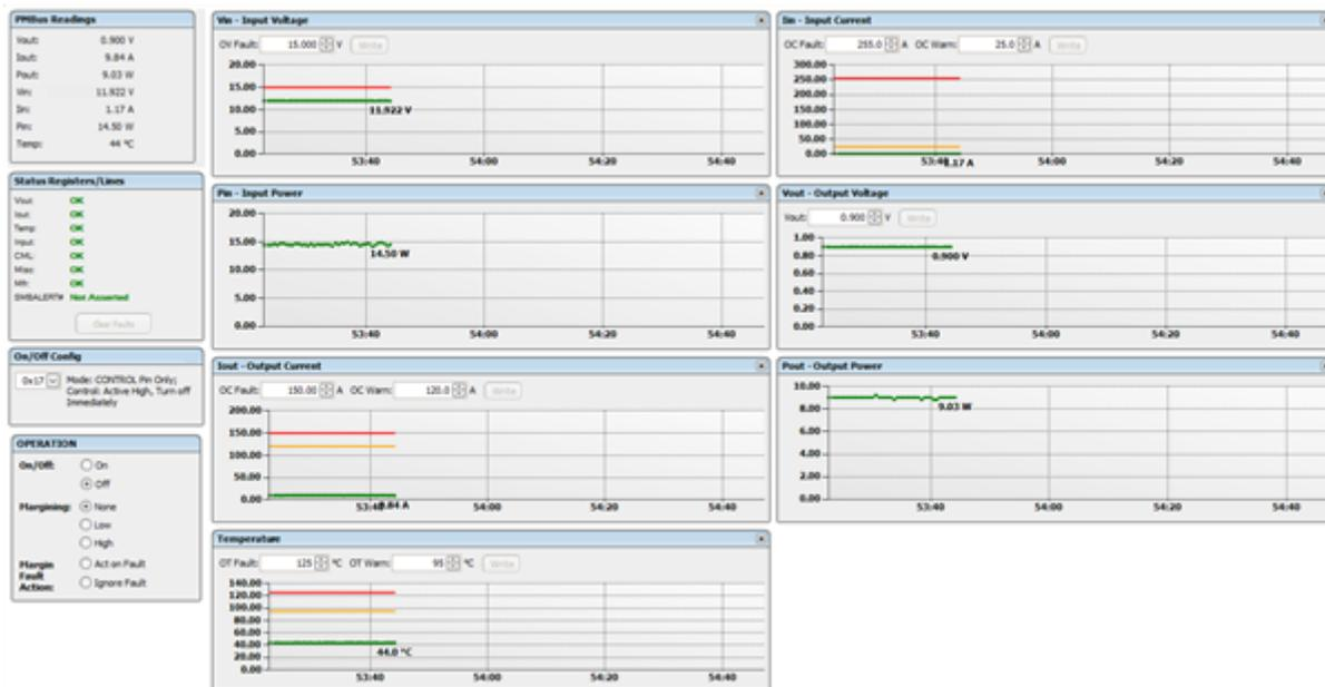
Figure 6. Input/output Voltage, Current, Temperature and Power through TI's PMBus Fusion Graphical User Interface (GUI) (TPS53647 Example)
