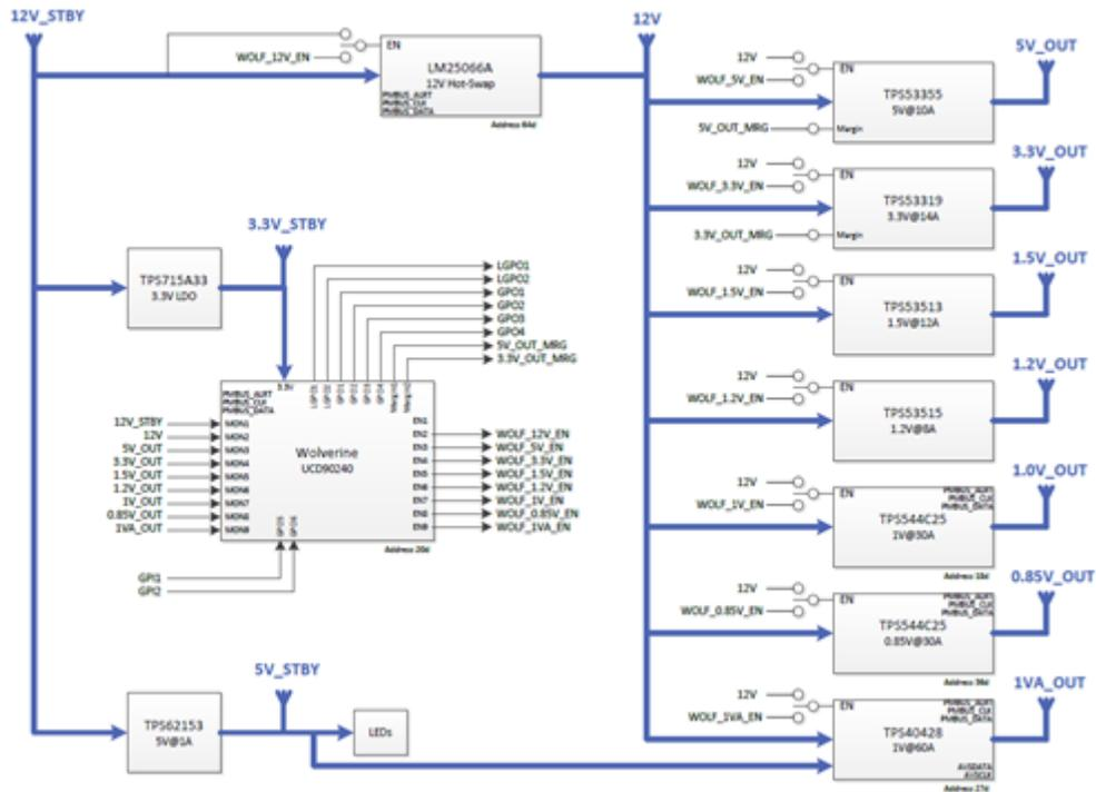
**Figure 4. PMBus Power System with PMBus Manager/sequencer and Analog and PMBus Voltage Regulators**
