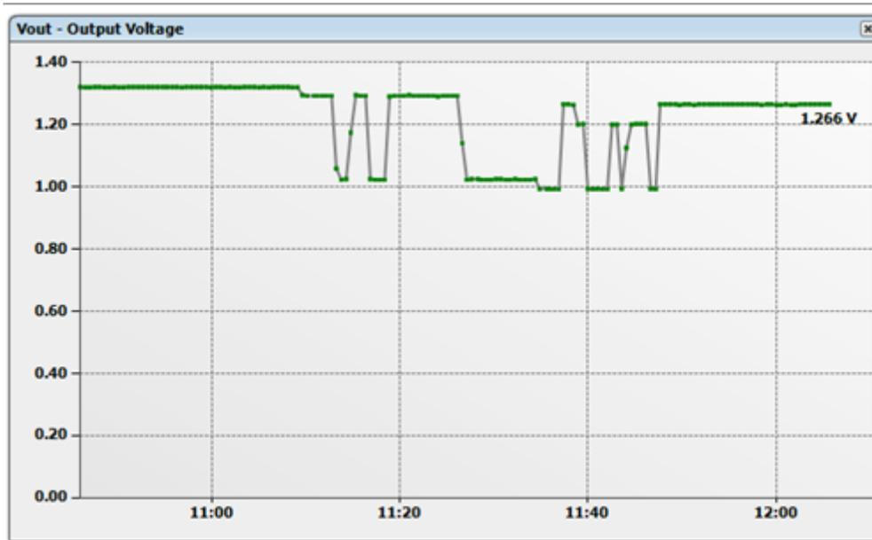
Figure 2. Output-voltage Margining through PMBus
