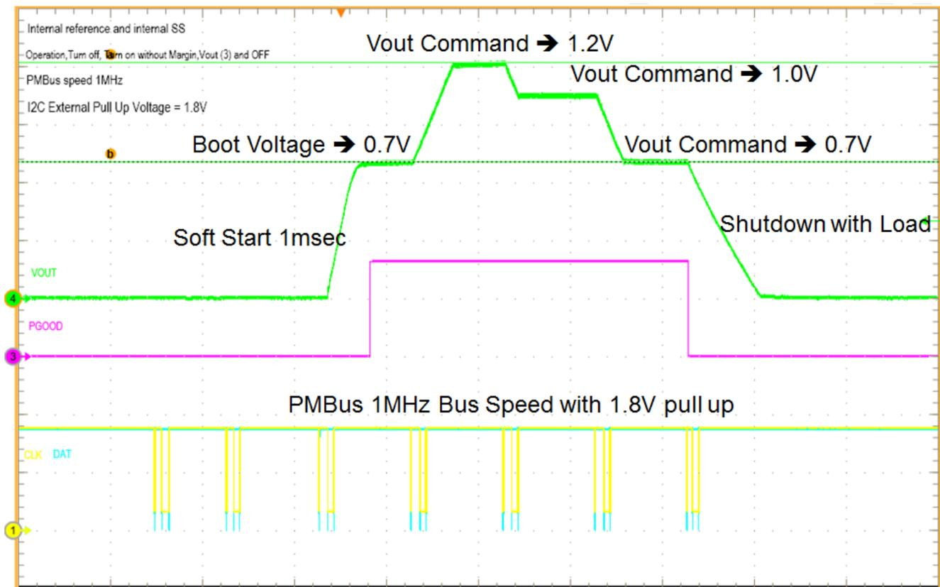
Figure 1. Output-voltage Adjustment through PMBus
