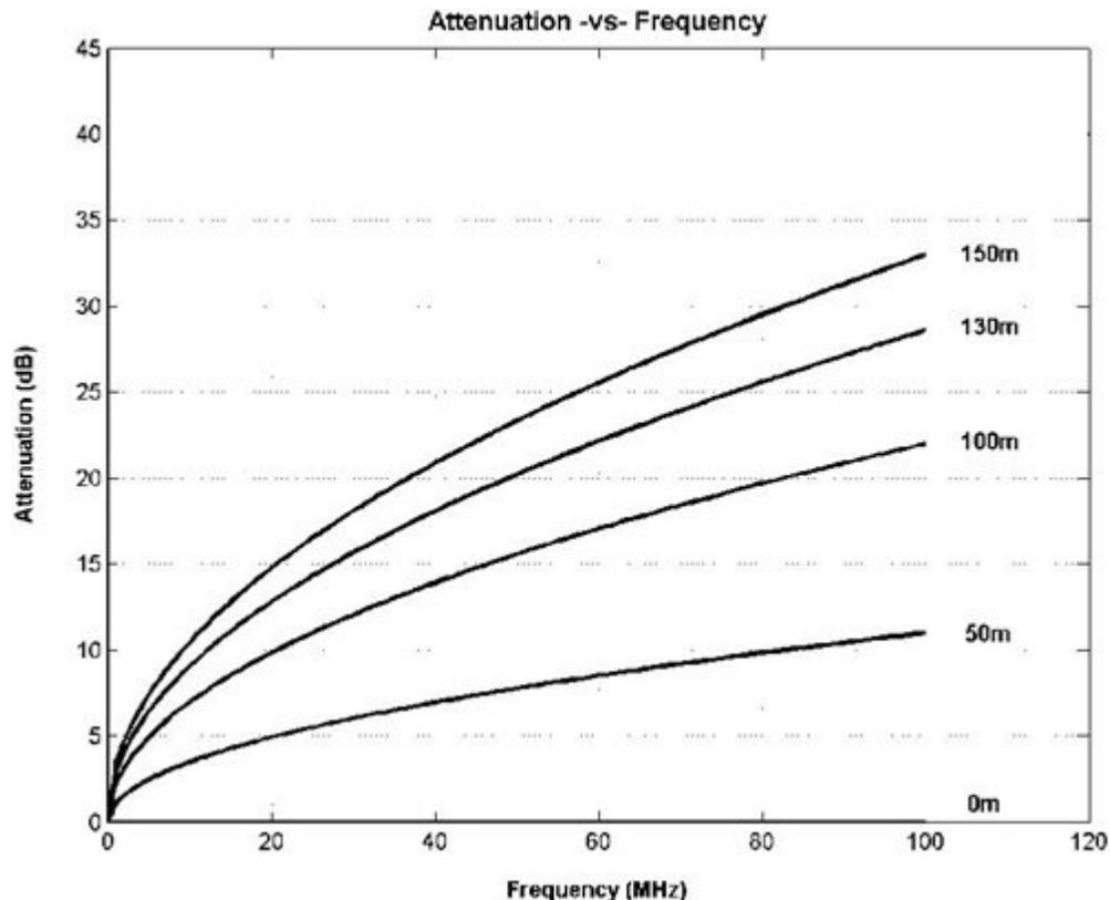
**Figure 1. Electronic Industries Alliance / Telecommunications Industry Association (EIA/TIA) Attenuation vs. Frequency for CAT 5 Cable**
