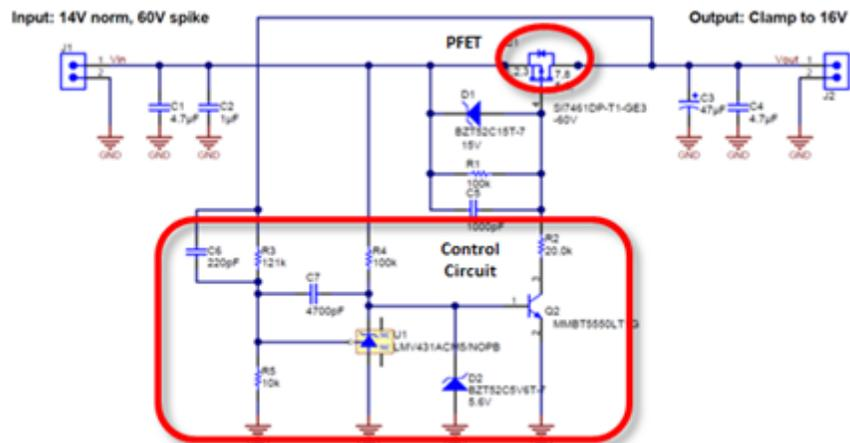
Figure 1. Discrete Solution Used to Clamp the Input Voltage
