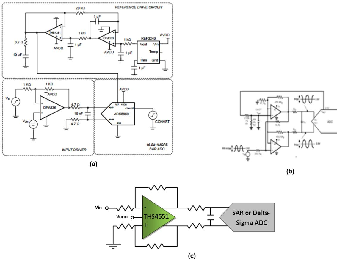
The FDA architecture can help significantly lower total harmonic distortion (THD) by reducing HD2. Implementing the FDA method shown in Figure 1c, you can achieve an improvement of >4dB in THD. This >4dB improvement can result in an overall system performance improvement, or give you the flexibility to use a lower-power/lower-bandwidth amplifier to meet the same THD.
