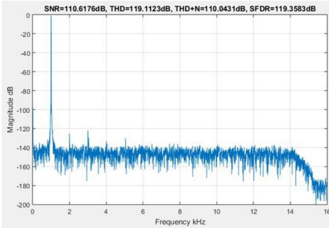
**Figure 4. ADS127L01 with THS4551 Spectrum**
