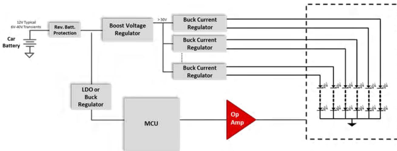
Figure 1. High-level System Block Diagram of LED Headlamp Lighting
