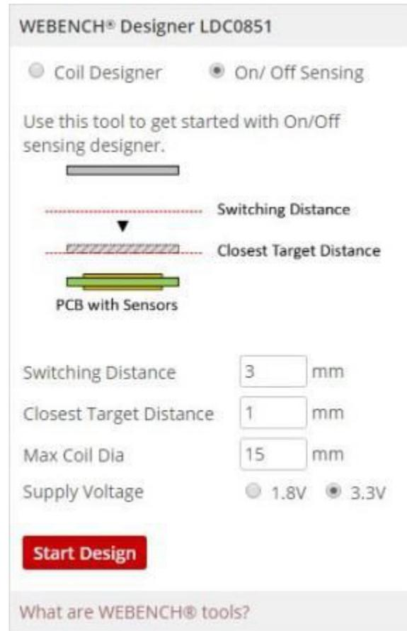
**Figure 2. Inductive Sensing WEBENCH Tool for Proximity-switch Applications**
