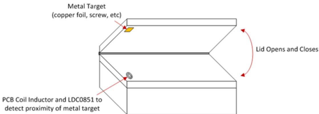
**Figure 1. Lid Open and Close Detection with LDC0851**
