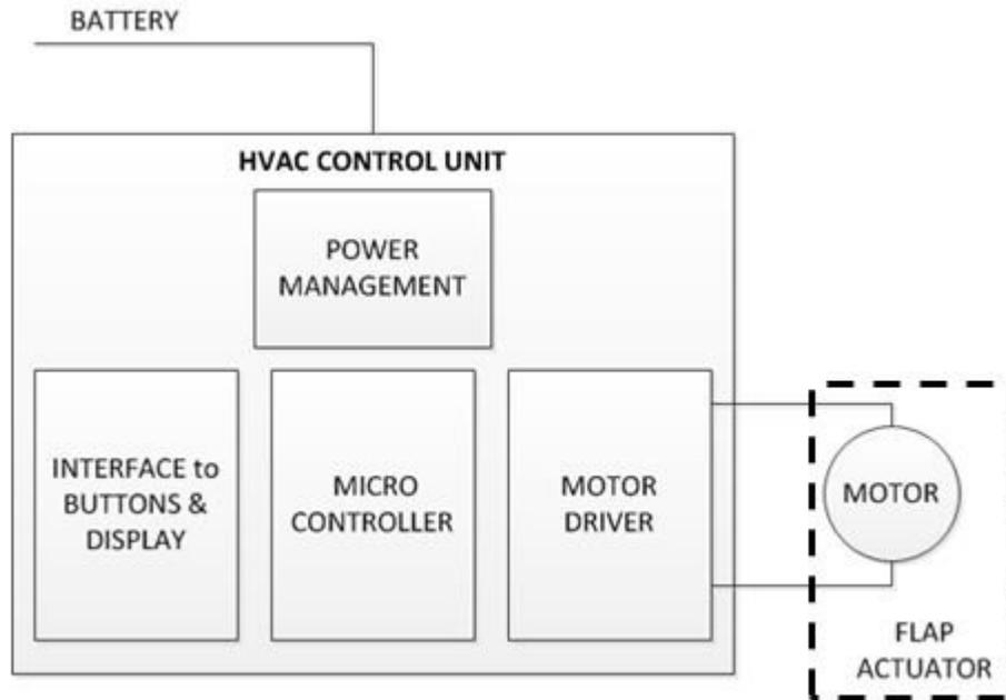
**Figure 3. Integrated Motor Driver for Flap Actuator**
