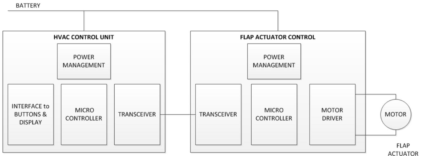
**Figure 2. Remote Control of Flap Actuator Motor**
