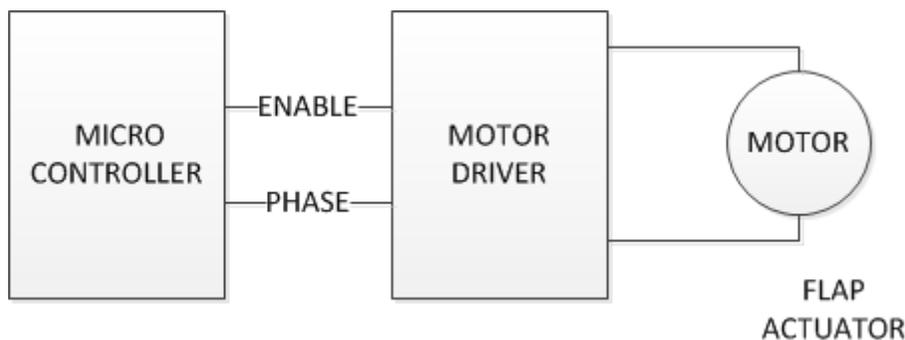
**Figure 5. A Microcontroller Controlling the Motor Driver Directly**
