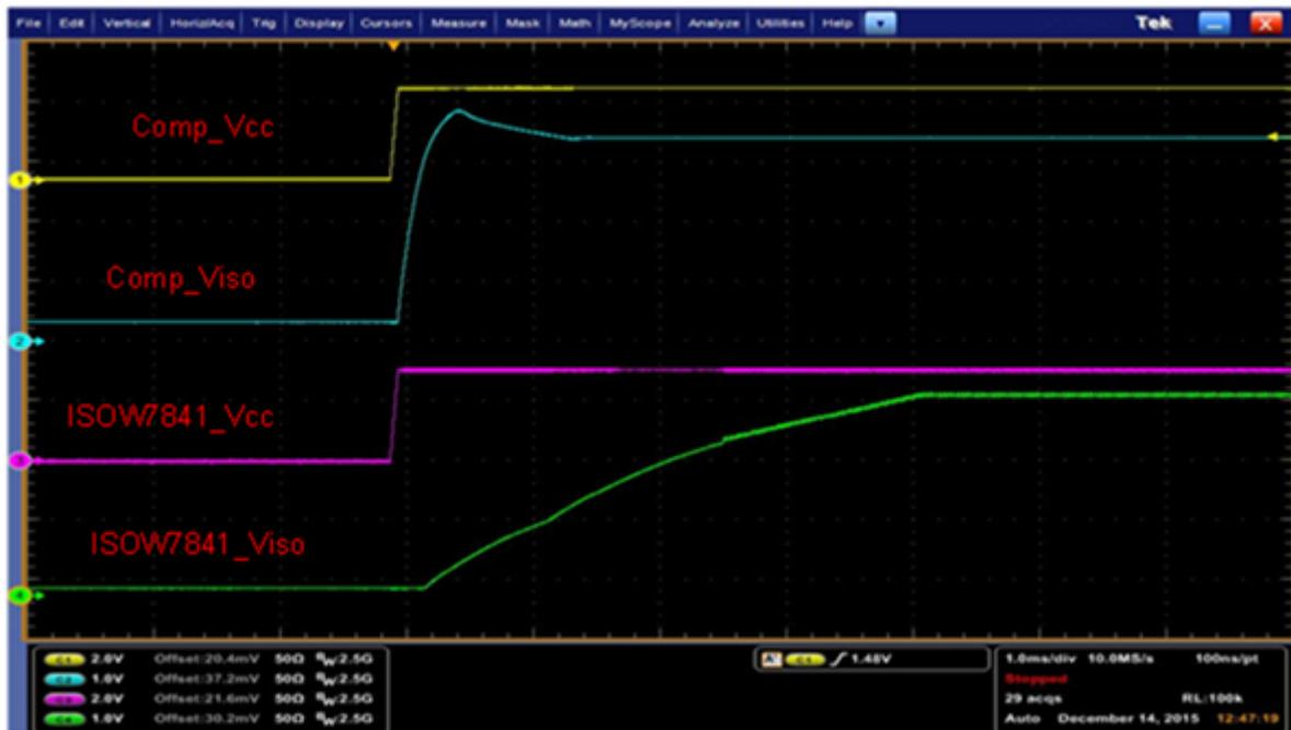
**Figure 5.  $V_{ISO}$  Power-up Oscilloscope Capture Compares  $V_{ISO}$  Waveforms of the ISOW7841 with a Similar Device on the Market**
