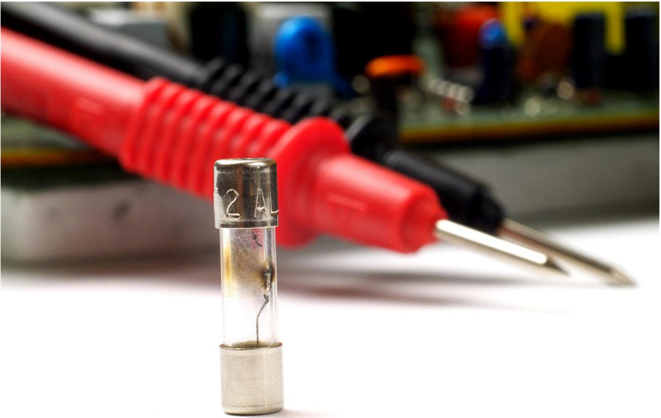
**Figure 2. A Blown Fuse Not Only Incurs Its Own Replacement Cost, But Also Could Be Responsible for Damaging Additional Components During the Overload Event Which Also Need to Be Replaced**
