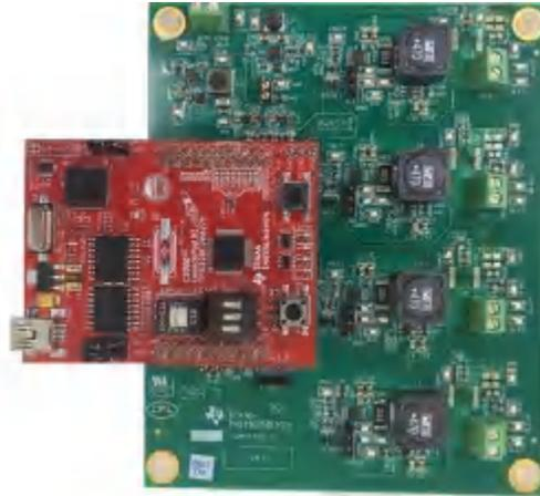
**Figure 2. Color-tunable Dimmable RGBW LED Luminaire Reference Design**
