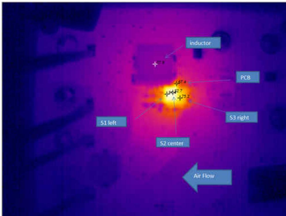
Figure 3. PCB with 35 Vias under the Thermal Pad
