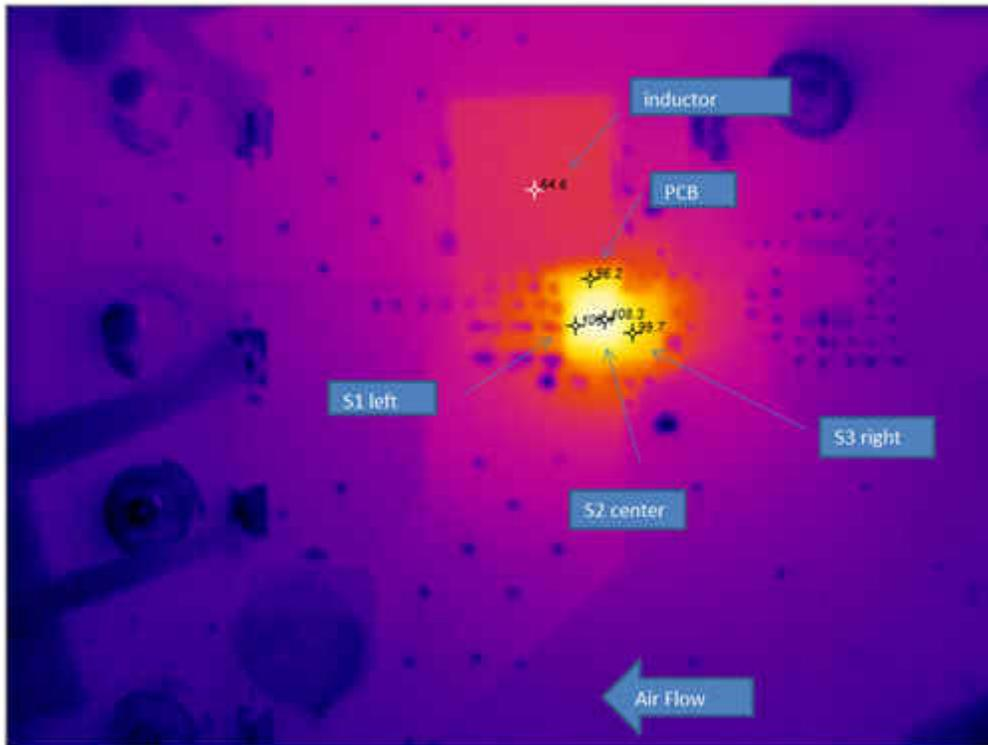
Figure 2. PCB with 11 Vias under the Thermal Pad
