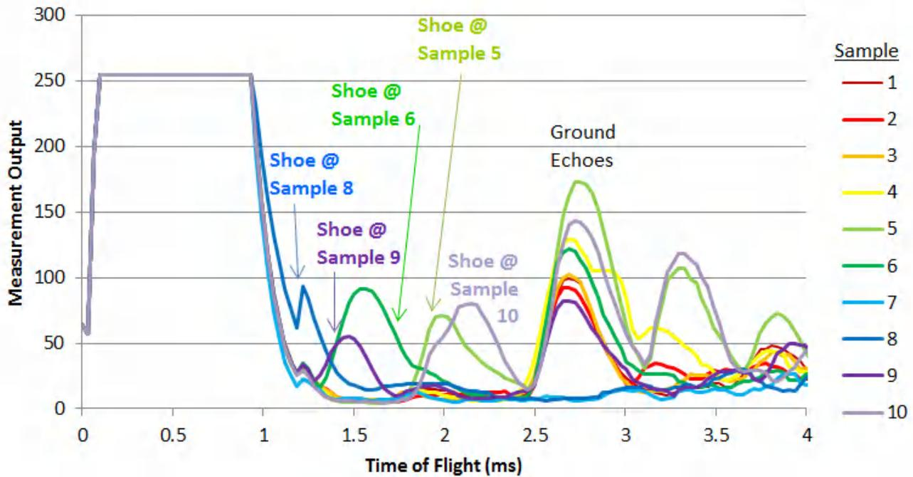
**Figure 2. Example Ultrasonic Sensor Response During Kicking Gesture**
