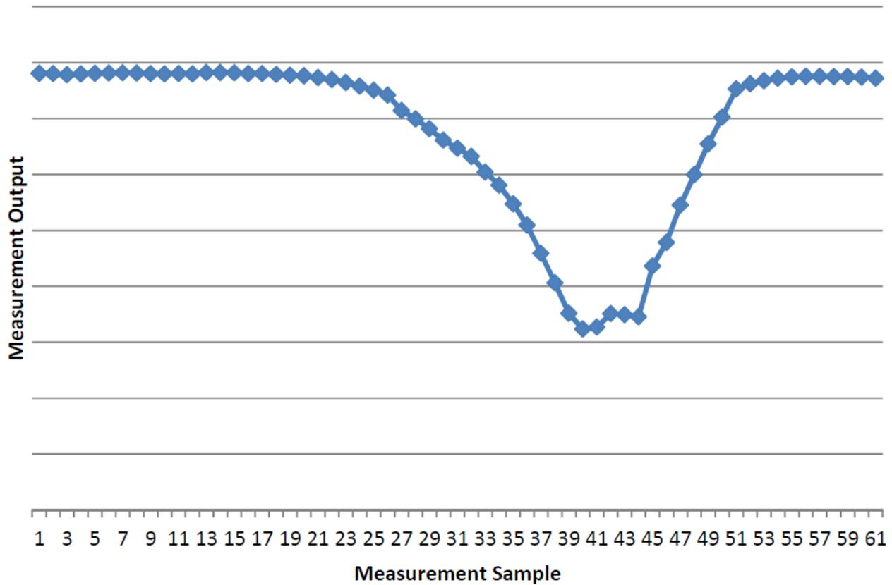
**Figure 1. Example Capacitive Sensor Response During Kicking Gesture**
