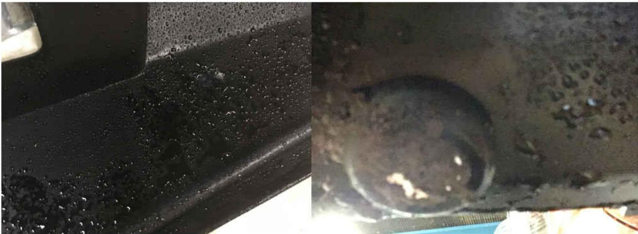
**Figure 3. Water on Capacitive Sensor, and Mud on Ultrasonic Sensor**
