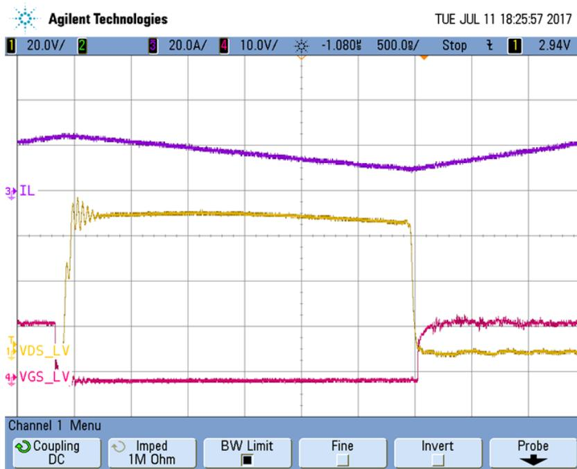
**Figure 2. Low Voltage MOSFET Turn on at ZVS**
