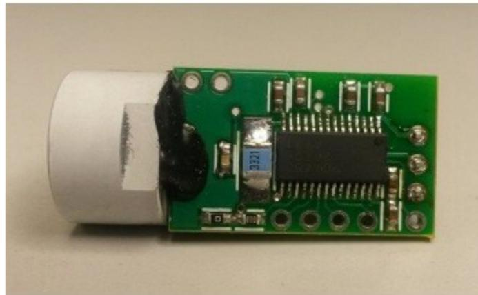
**Figure 2. Small Form Factor Ultrasonic Sensing Module**
