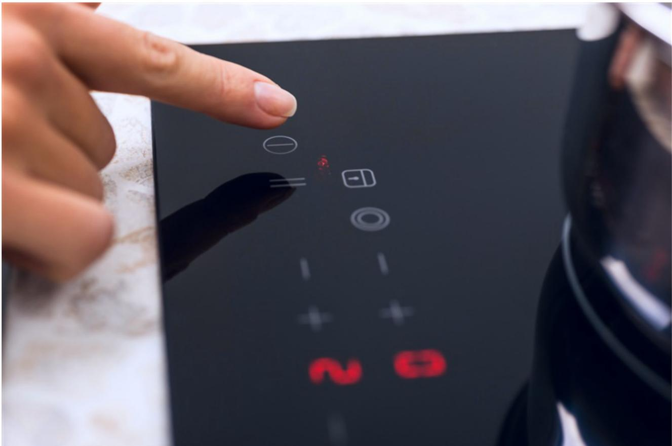
**Figure 1. Cooktop Controls Using Capacitive Touch**
