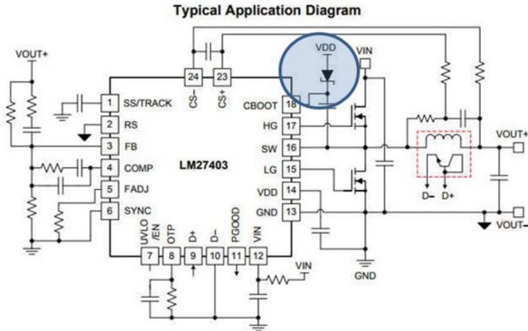
Figure 2. Application Circuit Showing VDD
