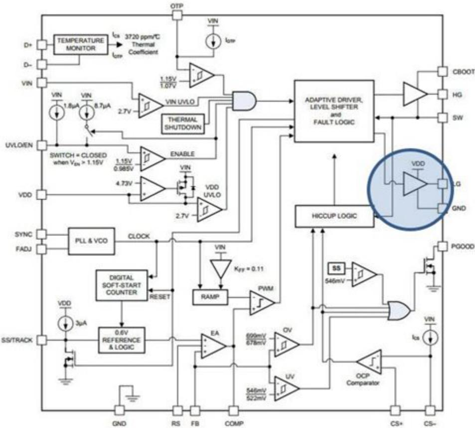
Figure 1. Block Diagram Showing VDD
