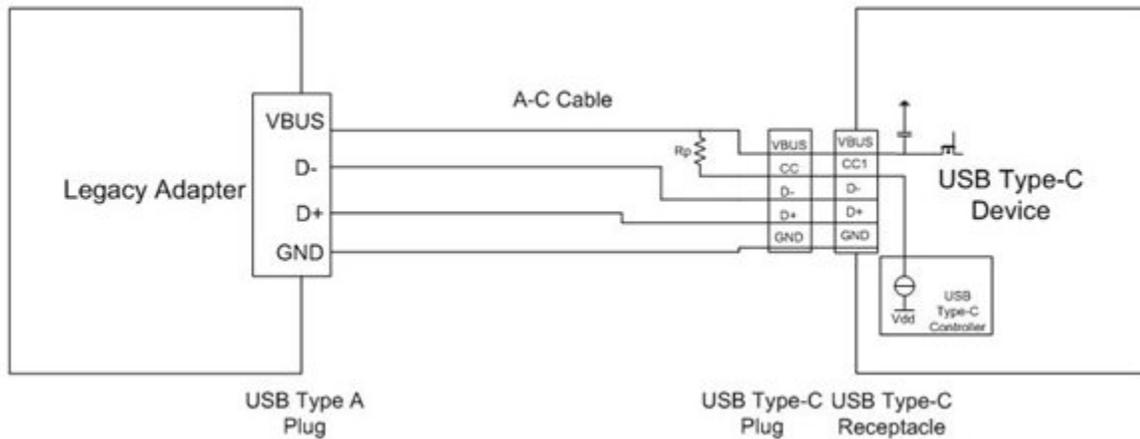
**Figure 2. Legacy Adapter to a USB Type-C Product Connection**
