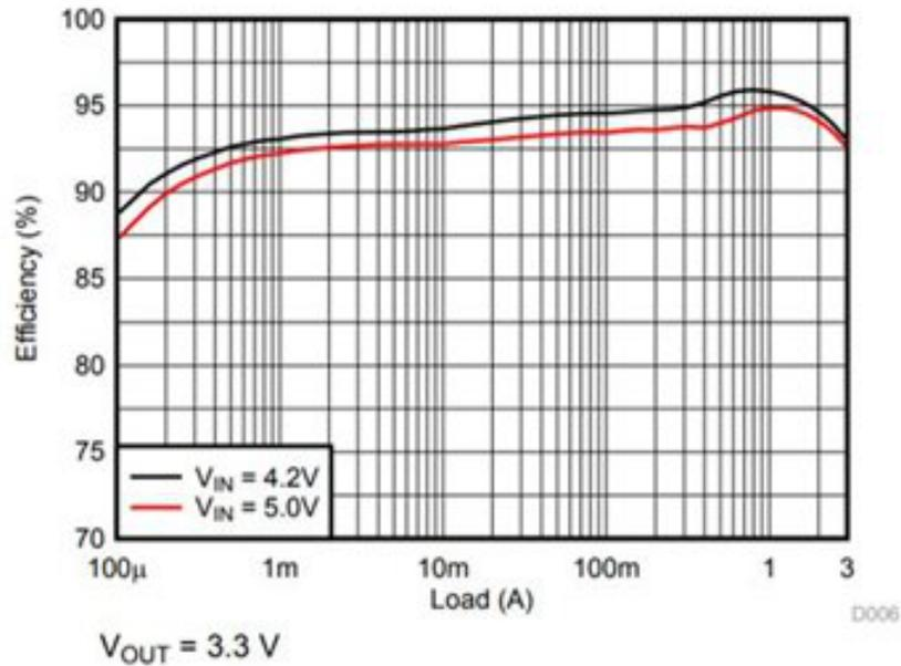
**Figure 4. TPS62088 Efficiency Is over 90% across the Entire Load Range**
