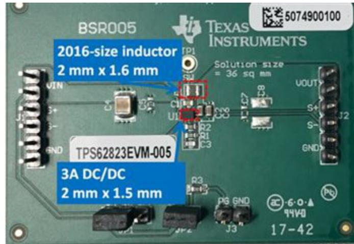
**Figure 2. A 3A DC/DC Is Smaller than a 2016-Size Inductor**
