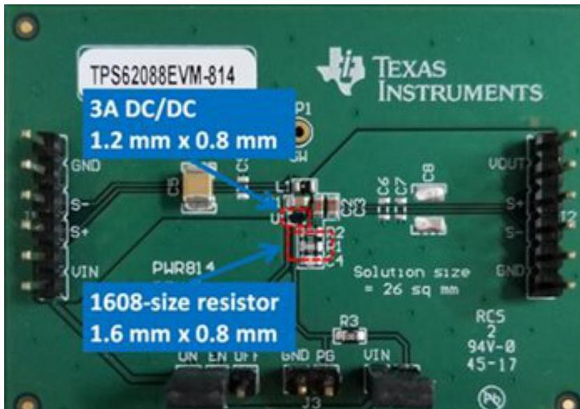
Figure 1. A 3A DC/DC Is Smaller than a 1608-Size Resistor
