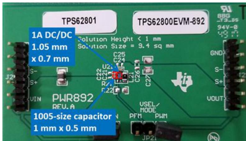
**Figure 3. A 1A DC/DC Is Almost as Small as a 1005-Size Capacitor**
