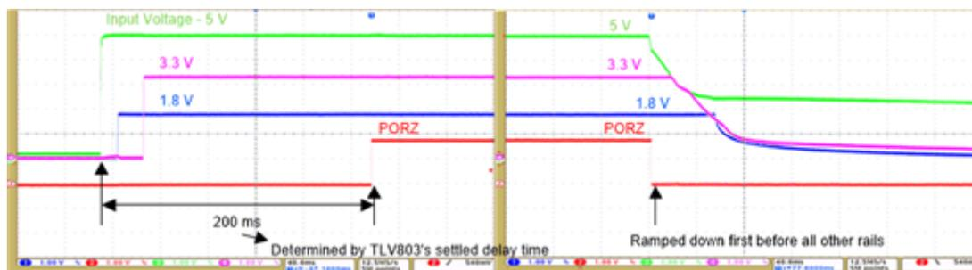
**Figure 3. Power Sequencing Test Result**
