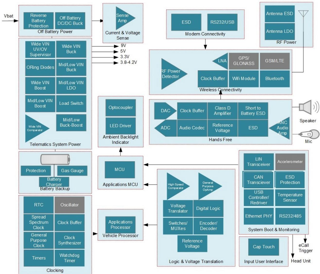
**Figure 1. Integrated Emergency Calling in a Modern-day TCU**
