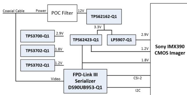
**Figure 2. Example of the Discrete Approach with the Automotive 2-MP camera module reference design with MIPI CSI-2 video interface, FPD-Link III and POC**
