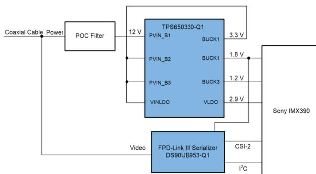
**Figure 1. Example of the Highly Integrated Approach with the Automotive Camera PMIC Power Supply Reference Design with Power Over Coax Filter**
