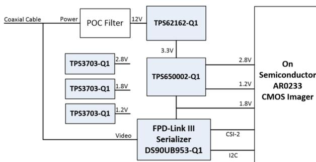
**Figure 3. Example of the Partial Integration Approach with Added Precision Diagnostics for the Supply Voltage Rails**
