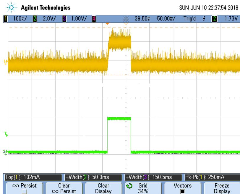
Figure 3. Pulse vs. Relay Current Waveform: Green Waveform = IN1; Yellow Waveform = Current across AOUT1 to AOUT2
