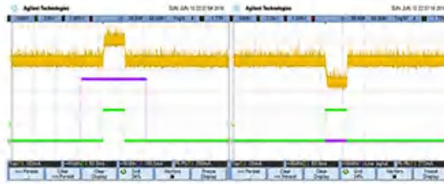
**Figure 10. Phase, Enable and Current through Relay Waveforms: Yellow = Current through Relay Coil (100 mA/div); Purple = Phase (1 V/div); Green = Enable (2 V/div)**
