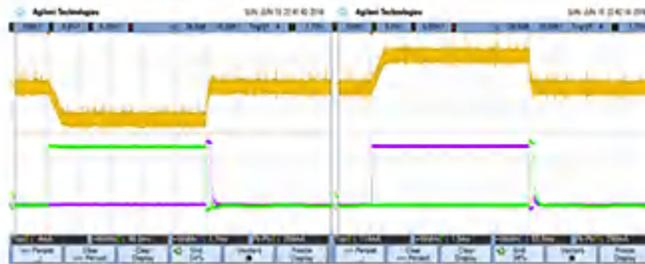
**Figure 11. OUT+ and OUT- and Current through Relay Waveforms: Yellow = Current through Relay (100 mA/div); Purple = OUT+ (5 V/div); Green = OUT- (5 V/div)**
