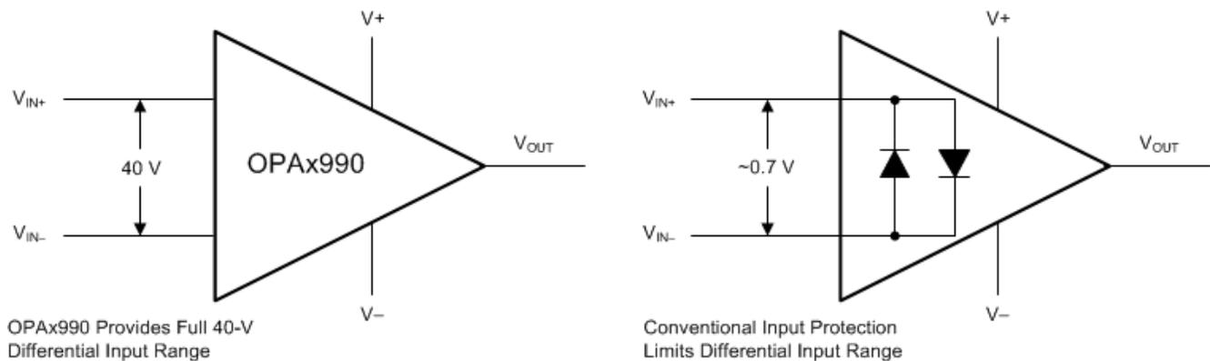
**Figure 4. OPA2990 Input Protection Does Not Limit Differential Input Capability (a)**
