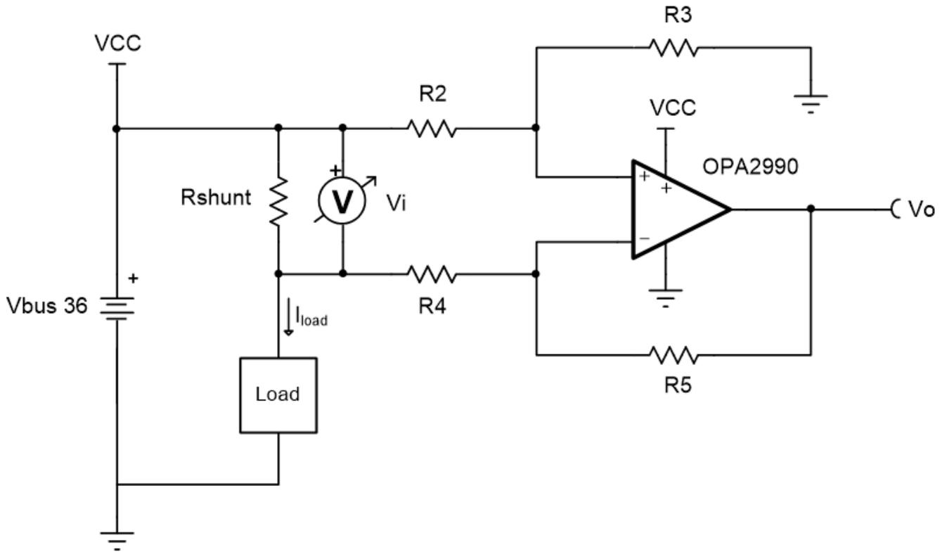
**Figure 2. High-side Current-sensing Circuit**
