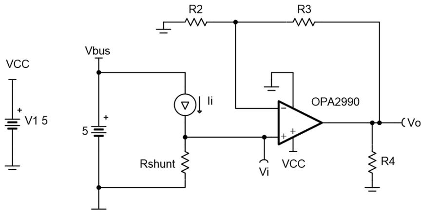
**Figure 1. Single-supply Low-side Unidirectional Current-sensing Circuit**
