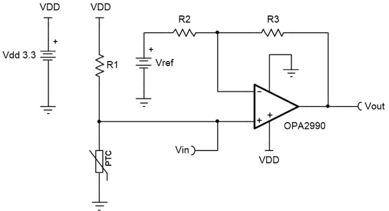
**Figure 3. Temperature Sensing with PTC Circuit**
