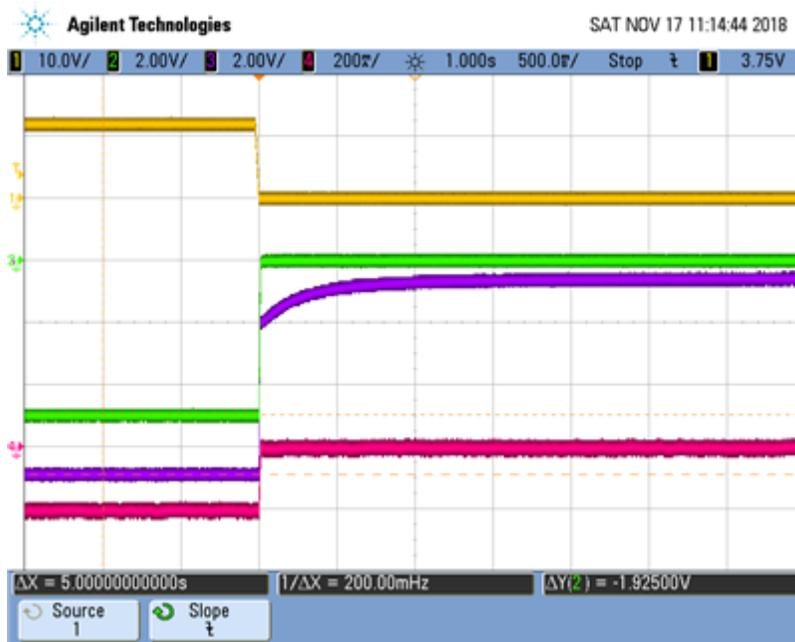
Figure 5. Shutdown Waveform for a 12-v Input at the DC/DC Converter (CH1 = VIN, CH2 = VOUTLDO, CH3 = VOUTDCDC, CH4 = IOUTLDO)
