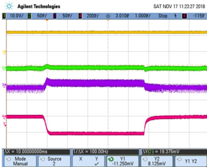
Figure 7. Load-transient Waveform at the Output of the LDO with a 200-mA Step Load (CH1 = VIN, CH2 = VOUTLDO [AC-coupled], CH3 = VOUTDCDC [AC-coupled], CH4 = IOUTLDO)
