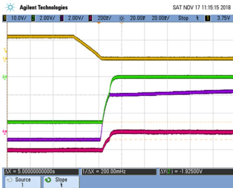
Figure 6. Zoomed-in Shutdown Waveform for a 12-v Input at the DC/DC Converter (CH1 = VIN, CH2 = VOUTLDO, CH3 = VOUTDCDC, CH4 = IOUTLDO)
