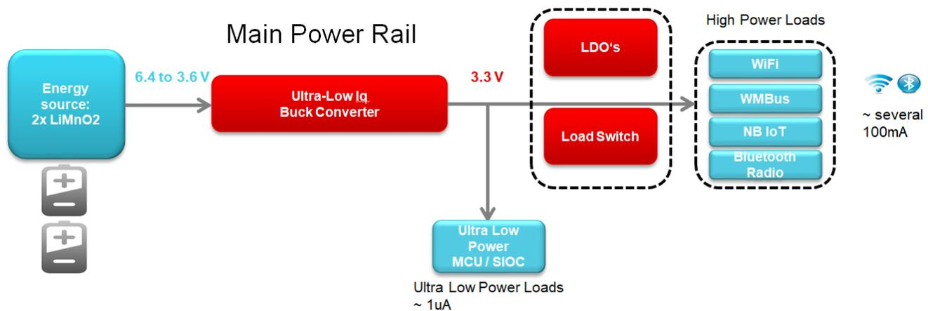
Figure 1. A Smart Meter Power Architecture
