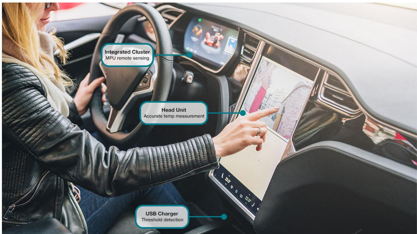
Figure 1. Infotainment and cluster systems where thermal issues are a key concern
