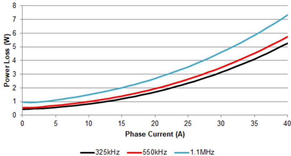
Figure 1. TPS546D24A power loss
