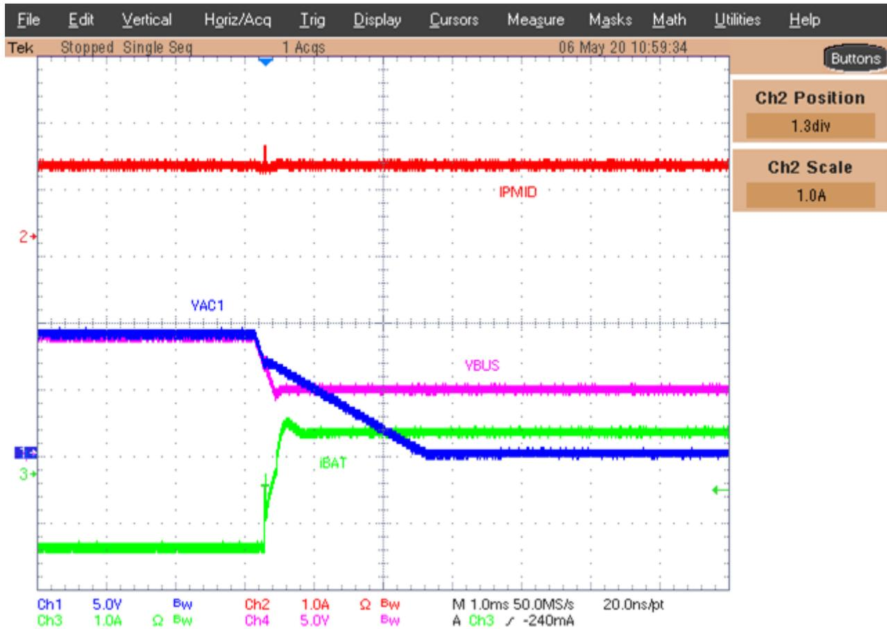
**Figure 4. Buck-boost charger FRS from  $V_{BUS}$  sink to  $V_{BUS}$  source.**
