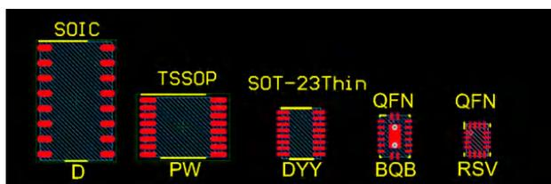
**Figure 2. TI 16-pin package footprint comparison**
