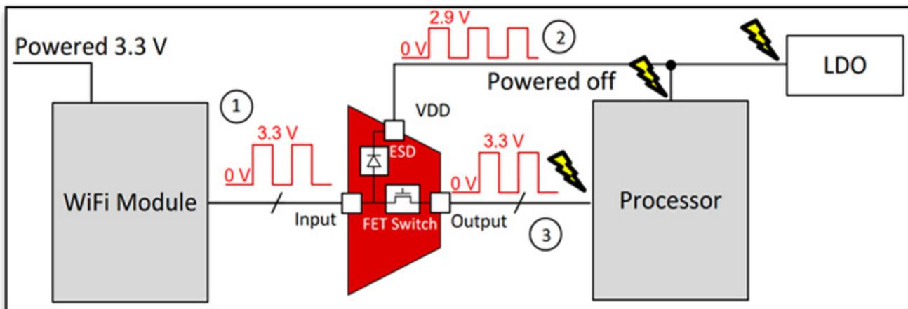
Figure 1. 3.3-V signal back-powering a multiplexer
