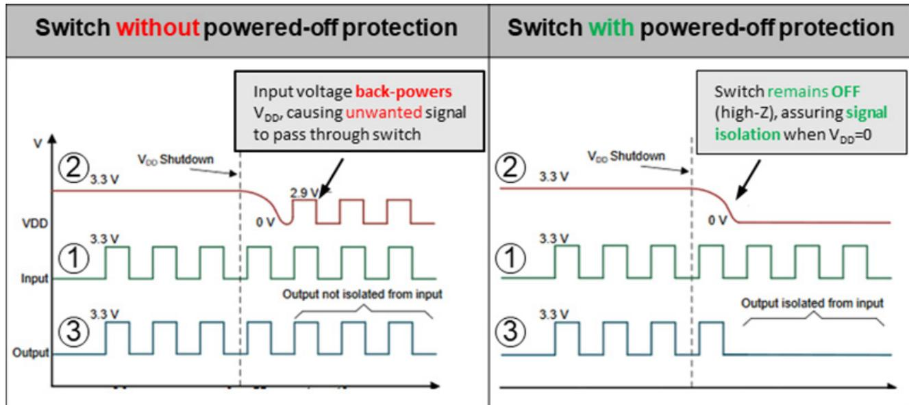
**Figure 2. Signal switch with and without powered-off protection**
